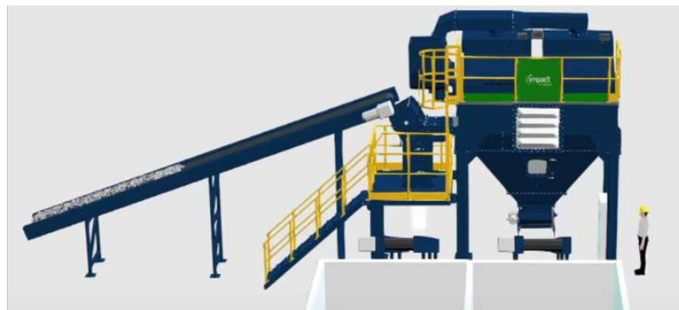
Image 16: Zigzag Air Classifier, provided by trial partner Impact Air Systems
