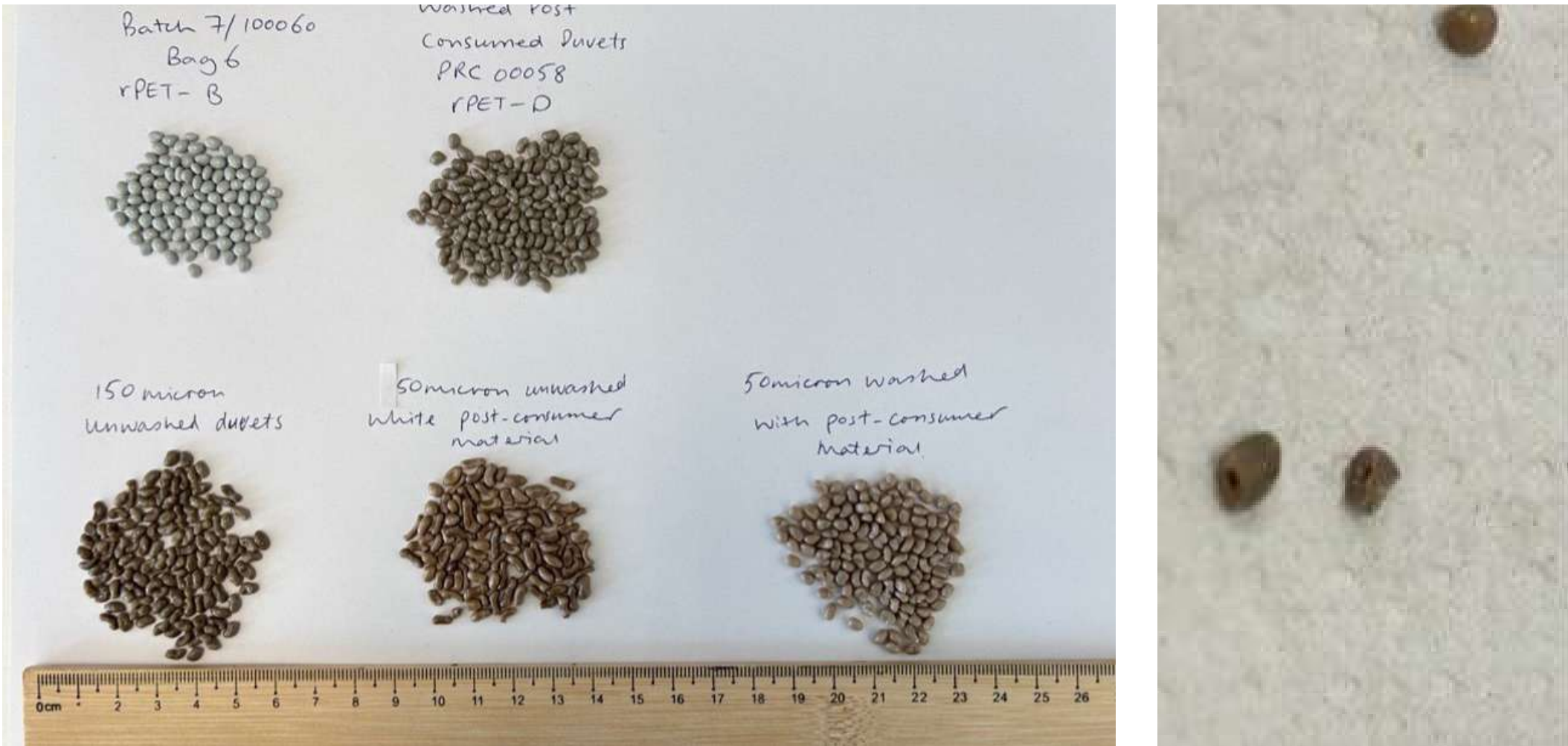
Image 24: Polyester Spinning Trial 1 PET pellets (left); Spinning Trial 1 hollow PET pellets (right)
