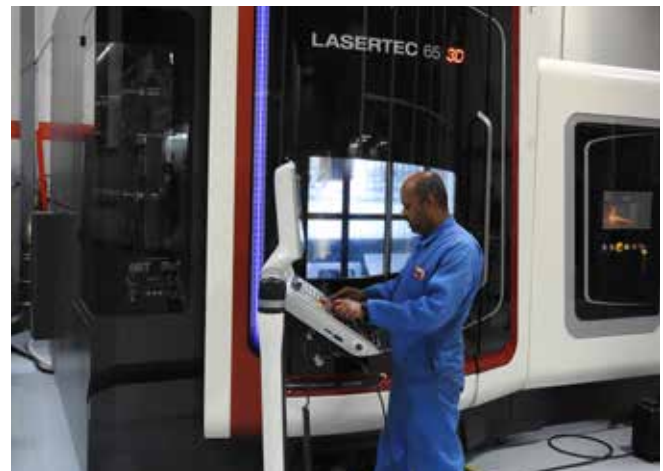
Romar is the only Australian company to offer a DMG MORI Lasertec 65 3D five-axis synchronous laser deposition, welding and milling machine.
