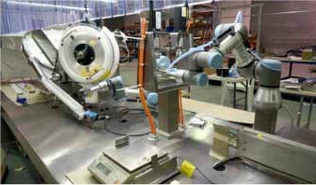
“We have completed handling, vision inspection, sorting, buffering and packaging systems for a range of products including syringes, vials and ampoules,” Hendy explains. “Also we have considerable experience in ampoule finishing processes including corona surface treatment (surface modification technique), pad printing, vision inspection, leak testing and serialisation.”
