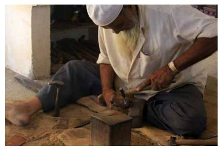
took a semicircular shape. The artist then employed a new tool – a metre-long iron rod with one pointed end and the other end bent to form a perpendicular shape with a flat top. He fixed the pointed end deep into the mud and over the flat top he positioned the semicircular iron scrap. After some more hammering and then cutting with scissors, the semicircle transformed into a hollow cylinder.
