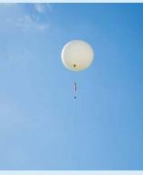
Weather balloons carry devices called radiosondes (middle) that are similar to the data-gathering sensors in the movie Twister. Weather balloons take flight from six National Weather Service offices in Texas.
