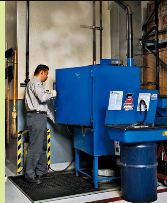
MOORE'S NEW PARTS-WASHING MACHINE IS BETTER FOR THE ENVIRONMENT AND HIS WORKERS — AND IS SAVING HIM MONEY ON SOLVENTS.
