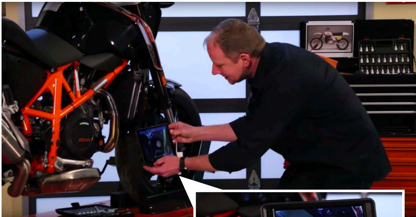
A KTM technician demonstrates how to visualize a malfunctioning motorcycle part on a tablet—and view AR instructions (green, in inset) on how to fix it,
