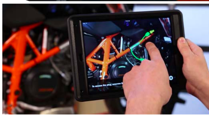
A KTM technician demonstrates how to visualize a malfunctioning motorcycle part on a tablet—and view AR instructions (green, in inset) on how to fix it,
