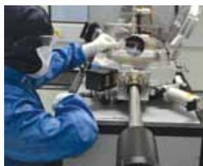
Thin-film deposition at MCN using atomic layer deposition.
