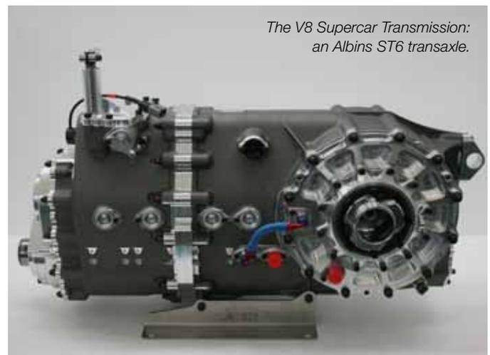
The V8 Supercar Transmission: an Albins ST6 transaxle.
