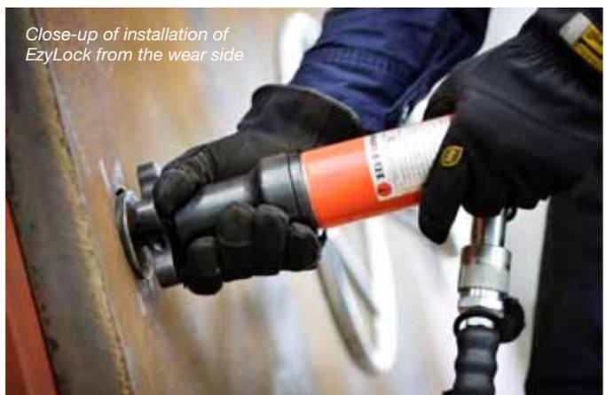
*Close-up of installation of EzyLock from the wear side*
