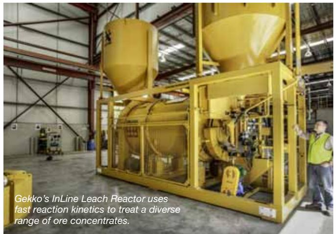
*Gekko's InLine Leach Reactor uses fast reaction kinetics to treat a diverse range of ore concentrates.*
