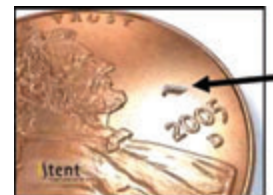
MIGS device on a penny shows scale.
