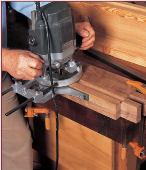
THE THREE COMPONENTS of the U-assembly are joined by finger joints. The slot cut out of the inner jaw in the foreground rides on the stationary teak guide bar.
