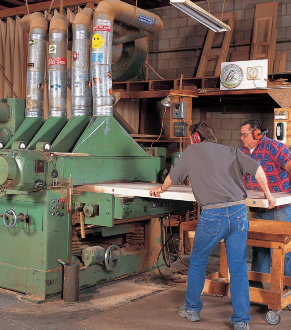
RUNNING A FULL-SIZE BENCH SLAB through a drum sander is a two-person operation; but it saves an enormous amount of time and effort, almost guaranteeing a perfectly flat benchtop.
