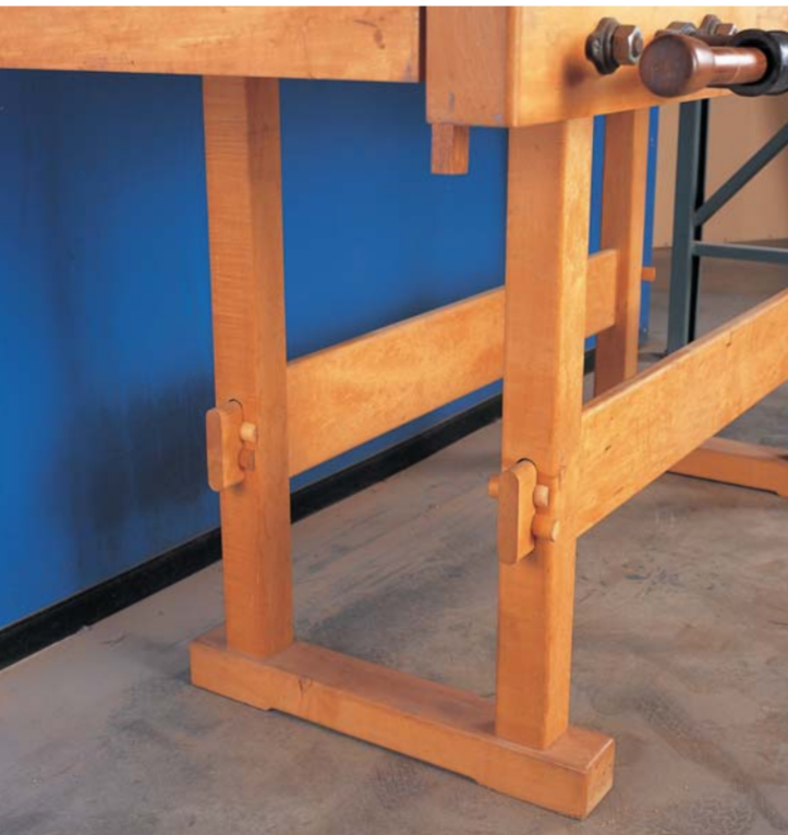
IN JOHN BARBEE'S CLASSIC ACORN BENCH , dowels flattened on one side act like wedges to pull the stretcher tight in the through-tenoned base.
