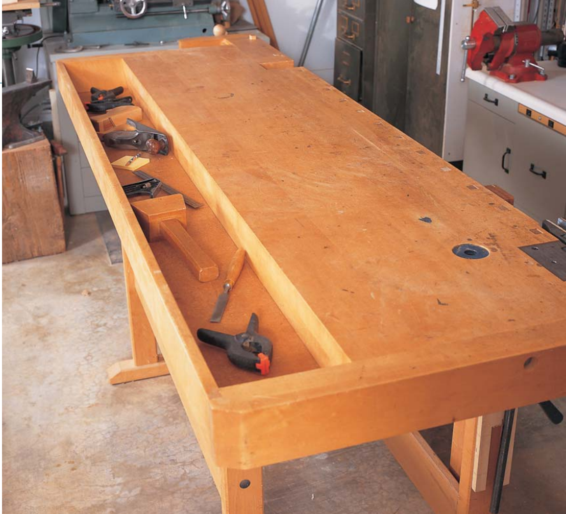
THE INTEGRAL TOOL TRAY on rear of this bench is the most typical configuration. The edge of the tray is usually at the same level as the bench surface, effectively increasing the useable area of the bench.
