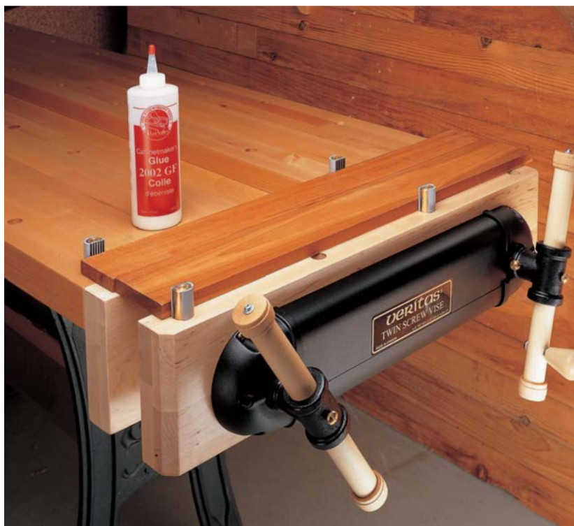
LEE VALLEY TOOLS' CHAIN-DRIVEN double-screw vise with its four bench dog positions can be used as a clamp for edge-gluing as well as for an end vise.
