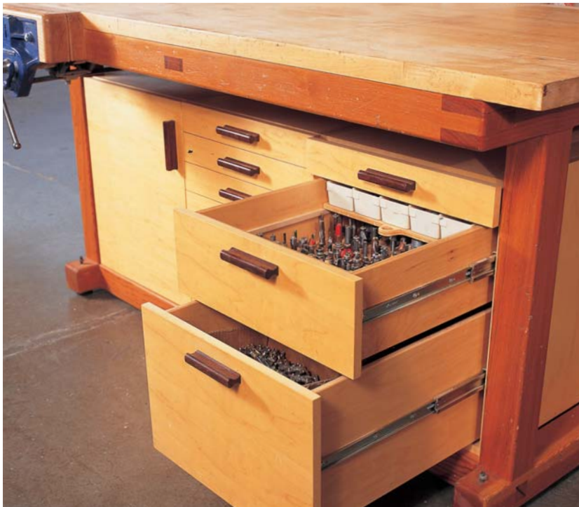
IN BRENT MERKLEY'S ROUTER BIT DRAWER, a sliding tray holds small plastic bins for storing small supplies and tools and keeps them organized and dust free.
