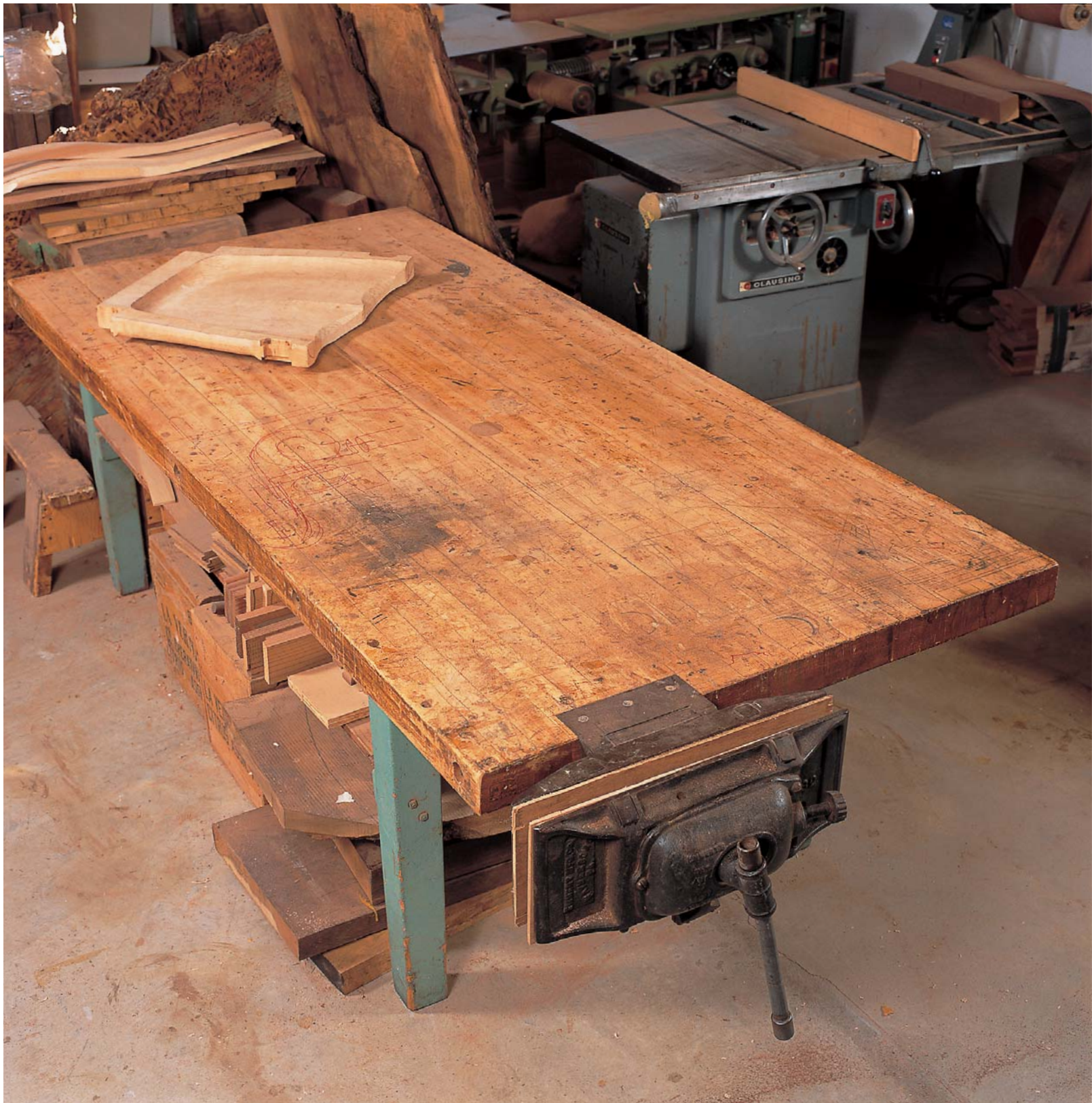
SAM MALOOF'S BENCHTOP , at 39 in. wide by 84 in. long, is on the larger side, but since he likes to work from both sides of the bench, it is narrow enough to easily reach to the center.
