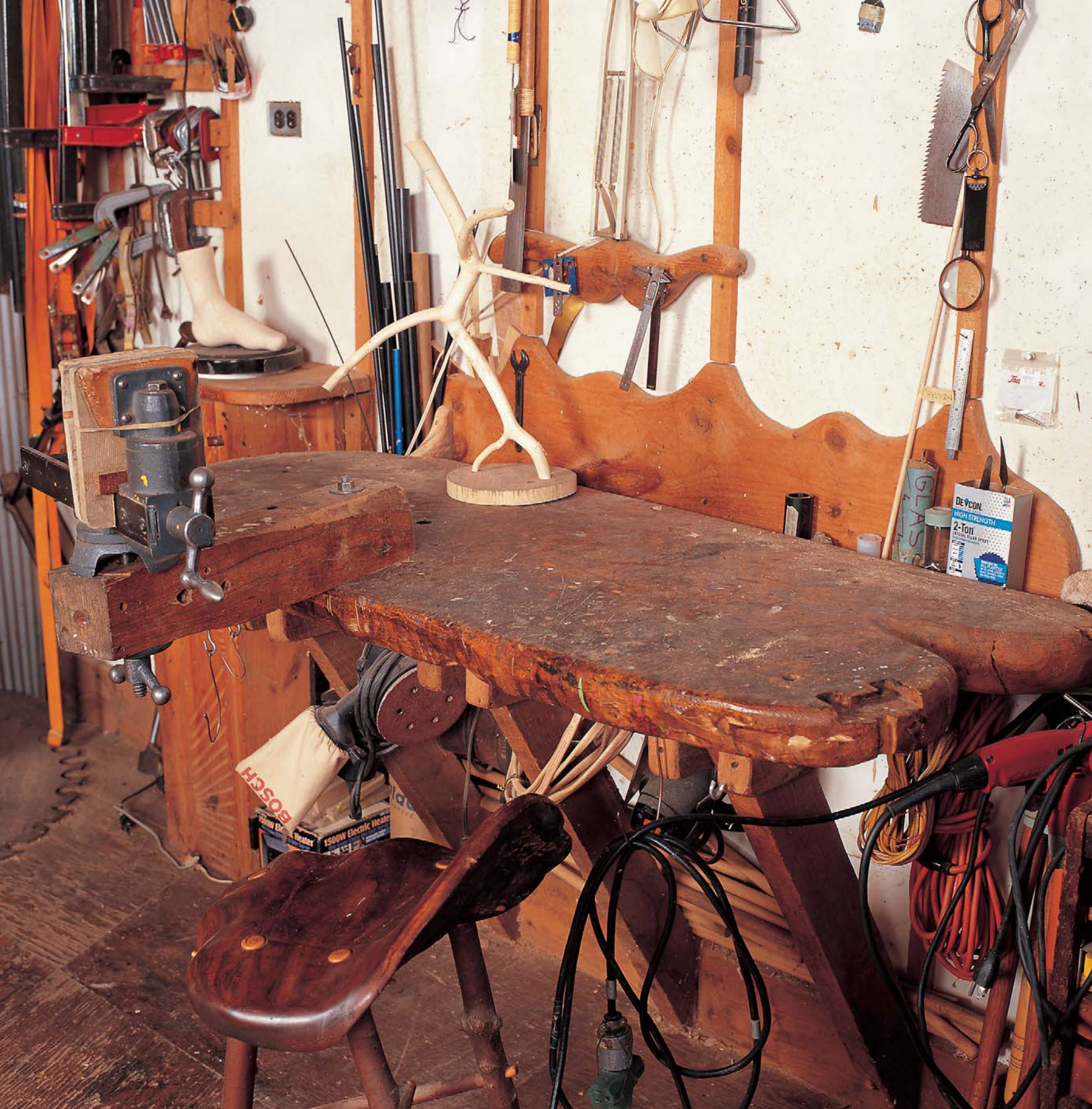
RUSTIC-FURNITURE MAKER JON BROOKS brought his craft to bench making. A solid-slab top holds a specialized vise, perfect for holding irregularly shaped parts.
