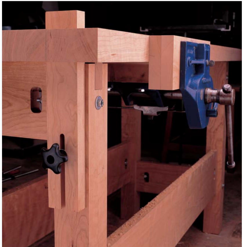
THE ADJUSTABLE POP-UP STOP is all Barrett needs to hold a board for handplaning. He can flip the board around quickly to reposition it or change direction without having to fumble with clamps or hold-downs.
