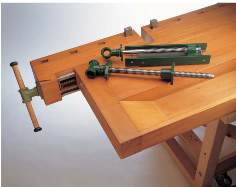
TWO TYPES OF TAIL VISE SCREWS. The top one has a steel housing. The lower screw is the type used with shop-built guides.
