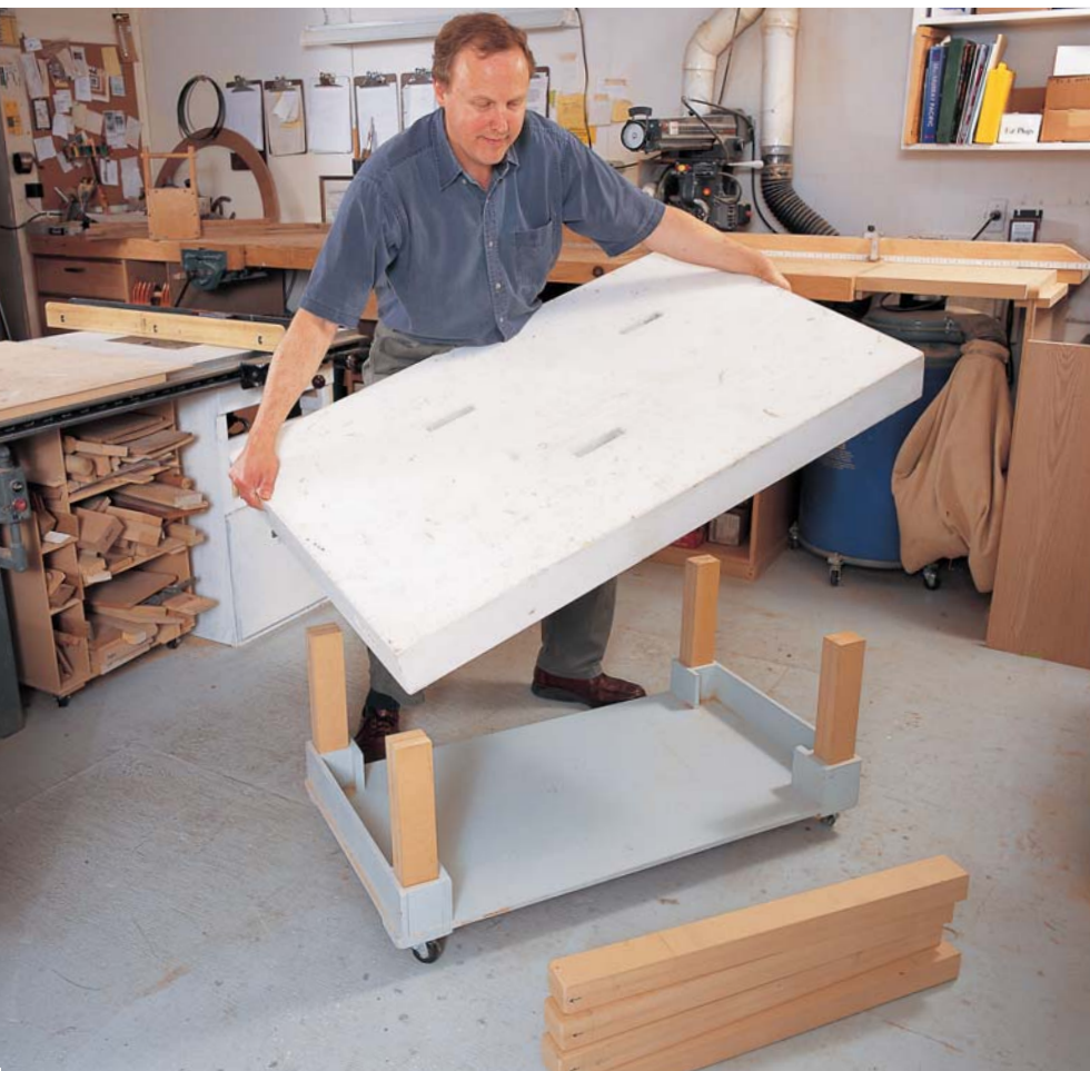
A TORSION BOX BENCHTOP is relatively light and easily lifted, so that John Weidner can interchange legs of different lengths. He can use the same base and benchtop as assembly table, rolling shop cart, or infeed table for his table saw.
