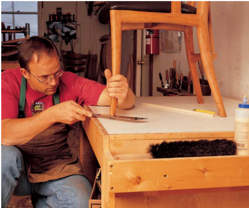
BRIAN BOGGS'S FINAL ASSEMBLY BENCH is a torsion box made perfectly flat. He uses it for, among other things, a platform to adjust the leg lengths of his famous chairs. He levels the chair and marks each leg for trimming. Once he's cut the legs to exact length, the chair sits flat without rocking.
