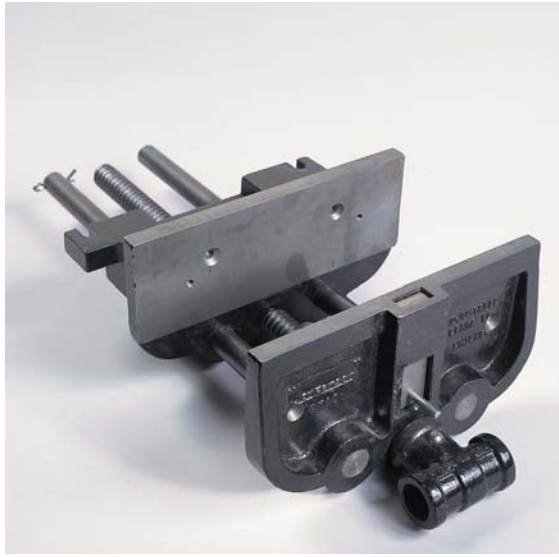
THE CAST-IRON JORGENSEN® VISE features quick-release convenience and pop-up bench dog. The quick-release mechanism uses a gravity-actuated half nut. Half a turn counterclockwise releases the jaw so you can slide it open or shut.
