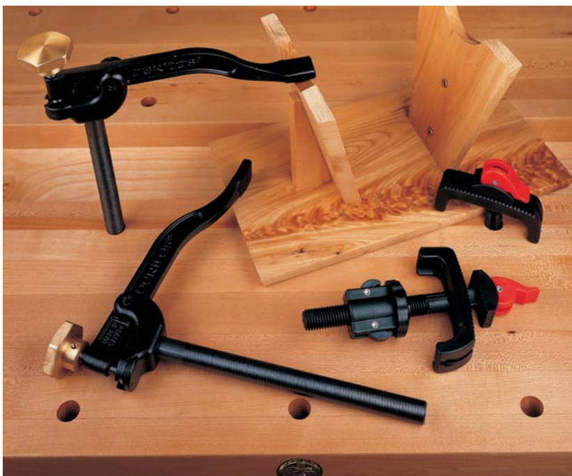
COMMERCIALLY MADE HOLD-DOWNS offer a reliable way to clamp boards to the surface of the bench. Benches with \frac{3}{4} -in. holes drilled for round bench dogs will usually accommodate a hold-down almost anywhere on the surface of the top.
