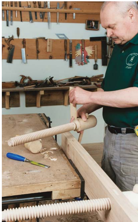
TEACHER AND WINDSOR CHAIR SPECIALIST MIKE DUNBAR chose wooden screws for the twin-screw front vise on his reproduction eighteenth-century workbench.
