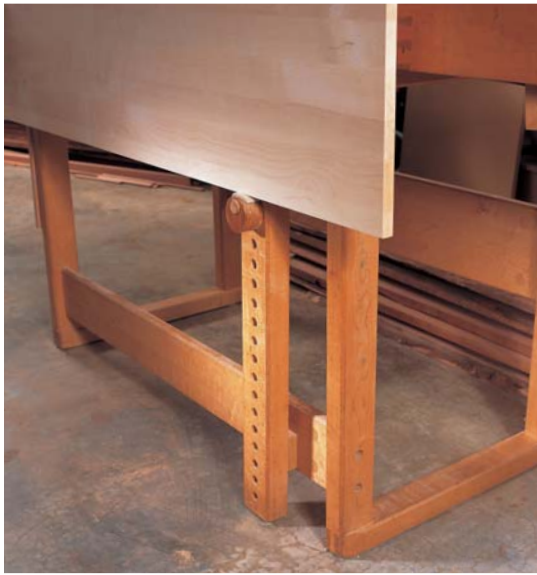
CURTIS ERPELDING'S BOARD JACK slides back and forth while suspended in a slot on the underside of the bench. He sets the height by inserting the round support in one of the holes; to fine-tune the height, he rotates the support.
