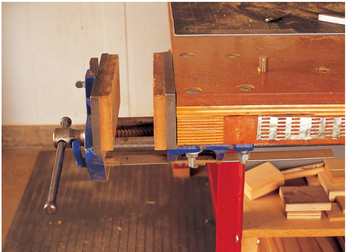
THE EASIEST VISE INSTALLATION is on a bench with a top that is just exactly thick enough to hold the jaws at the right height. With a thinner benchtop you'll have to add blocks below it. This vise is mounted proud, with the rear jaw beyond the front edge of the bench.
