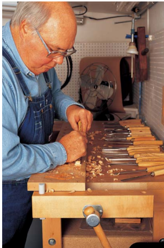
ROTATING ROUND DOGS ARE ESPECIALLY USEFUL for carvers, like Clyde Richardson, making it easy to hold irregularly shaped work.
