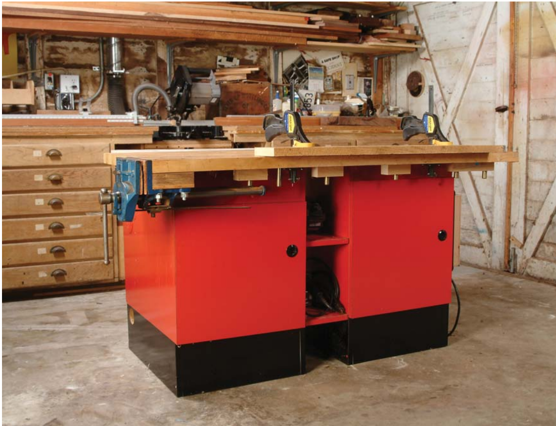
SANDOR NAGYSZALANCZY GATHERED THE PARTS OF THIS BENCH from a variety of sources. The assembly was a simple matter of bolting on a vise, drilling some dog holes, and screwing the top to the base cabinets.
