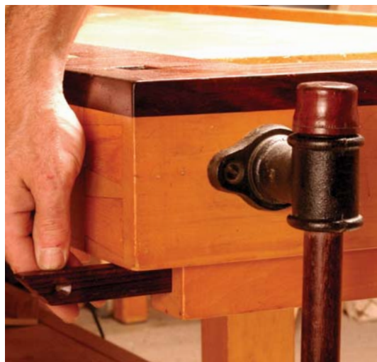
THIS HANDY PULL-OUT SUPPORT in Andy Rae's workbench is always available to hold a long workpiece for hand-planing. When not in use, the support disappears into a slot under the bench.
