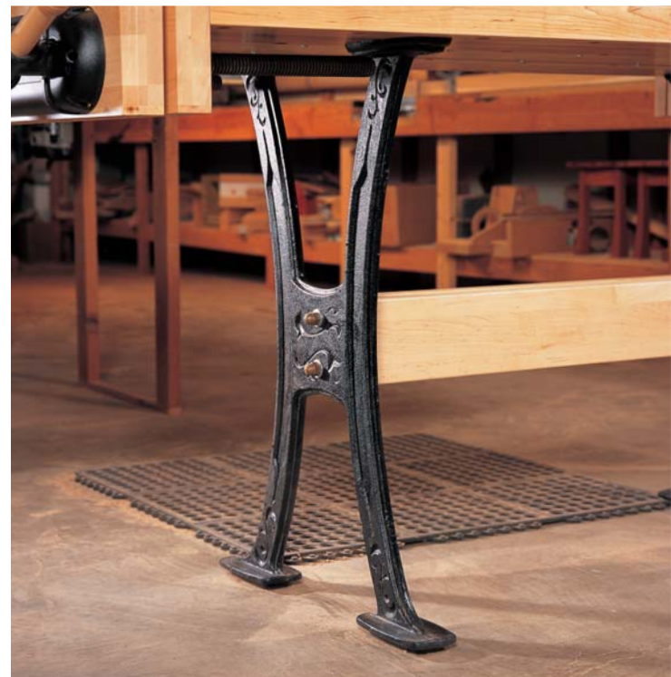
THESE CAST-IRON BENCH LEGS are reminiscent of the beautiful machines built in the nineteenth century. Not only are they elegant looking and absolutely rigid, they're heavy enough to provide good stability to any bench.
