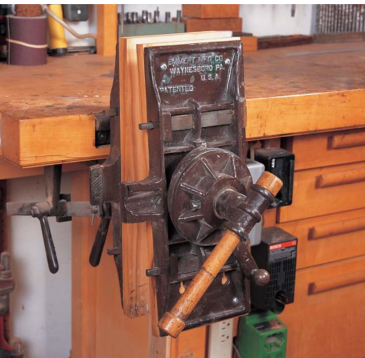
ROTATED VERTICALLY , this Emmert patternmaker's vise brings the workpiece above the level of the benchtop for detail work. Note that with the wooden pads installed, the small metalworking jaws won't close completely.
