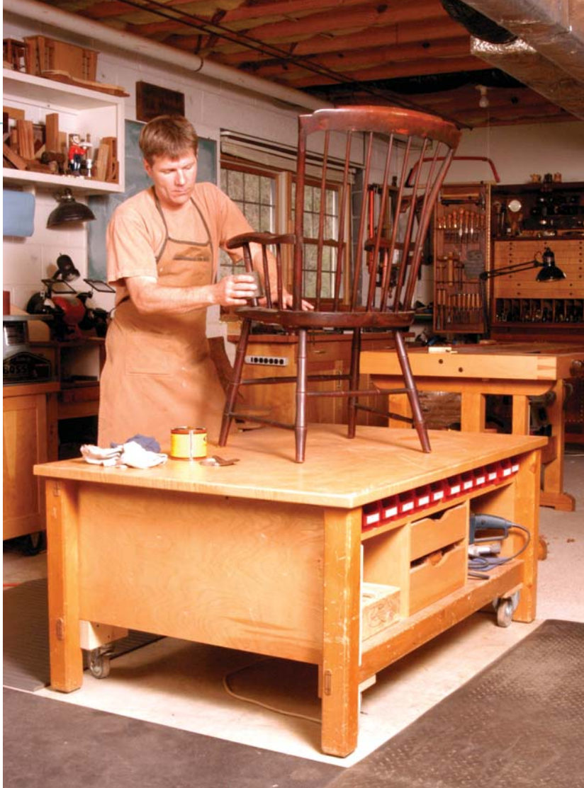
ANDY RAE'S LOW ASSEMBLY TABLE is at the perfect height for working on furniture. The bench provides a glue-up surface, a finishing table, a place to lay out parts, and storage for tools and supplies. It also helps keep the main bench uncluttered in his busy shop.
