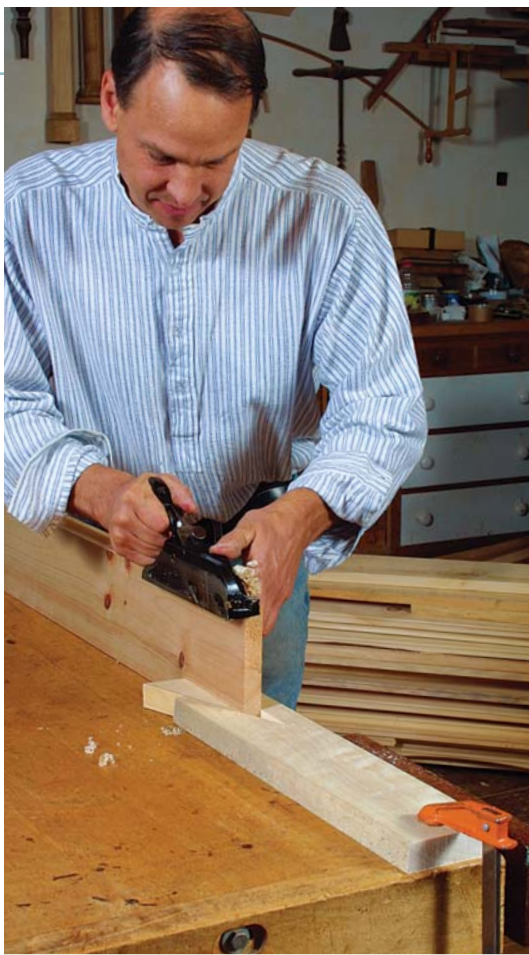
GARRETT HACK USES A BIRD'S-MOUTH STOP when planing a board on edge. The cutout created when making the stop is the perfect wedge for securing the work.
