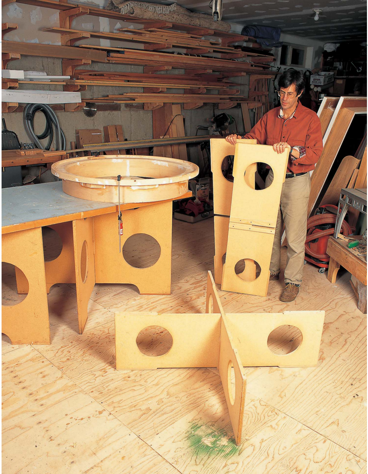
THESE STOW-AWAY BASES , built by woodworker and author Jim Tolpin are made from inexpensive particleboard reinforced with cleats where they connect. When not in use, the base and the top can be stored flat against the wall.
