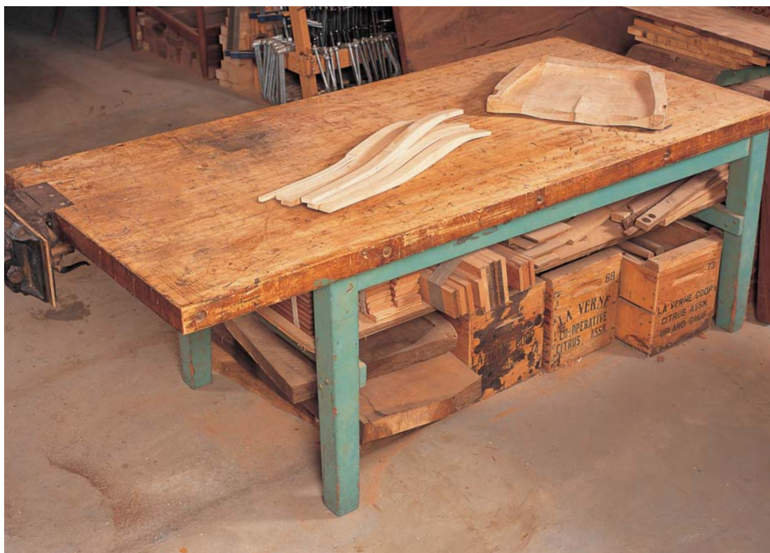
THIS BASE BUILT BY SAM MALOOF could as easily have been a leg-and-apron base for a dining table. By adding a cross brace between the legs, Maloof created a place to hold a useful under-the-bench shelf.
