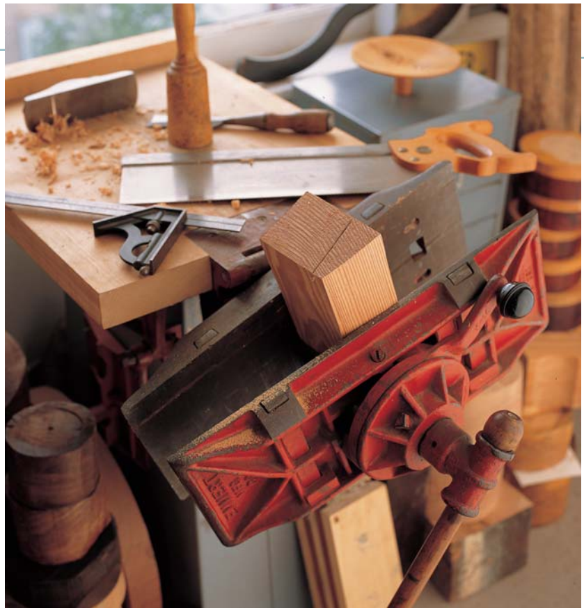
THE EMMERT NUMBER 1 UNIVERSAL is the larger of the two vises in this class. Its jaw capacity is 14 in. without pads. It's just about the perfect vise for working irregularly shaped parts.
