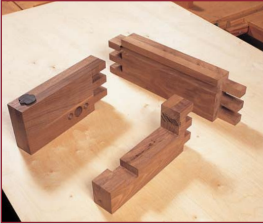
THE THREE COMPONENTS of the U-assembly are joined by finger joints. The slot cut out of the inner jaw in the foreground rides on the stationary teak guide bar.
