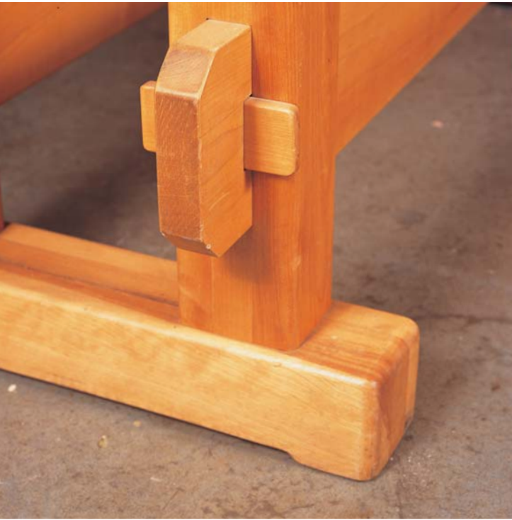
BRENT MERKLEY secured the through tenon with a cross-wedge. Pounding it in draws the parts together tightly.
