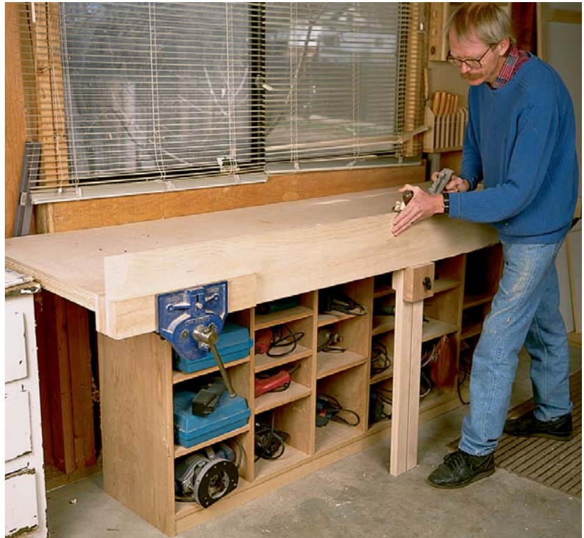
LARS MIKKELSEN MADE A BOARD JACK with a bracket at the top that locks into place with the bench dogs he makes from 1-in. dowels. The outer face of the leg is in the same plane as the inner jaw of the vise.
