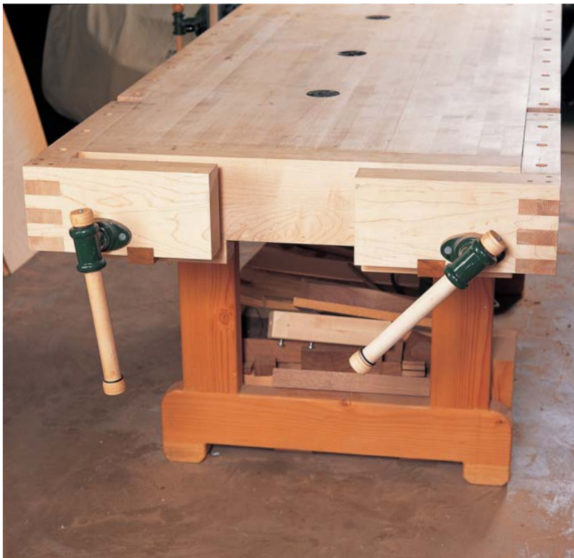
DOUG BETTS BUILT TAIL VISES on each corner of his bench. This way, depending on his inclination, he can use either hand or either side of the bench.
