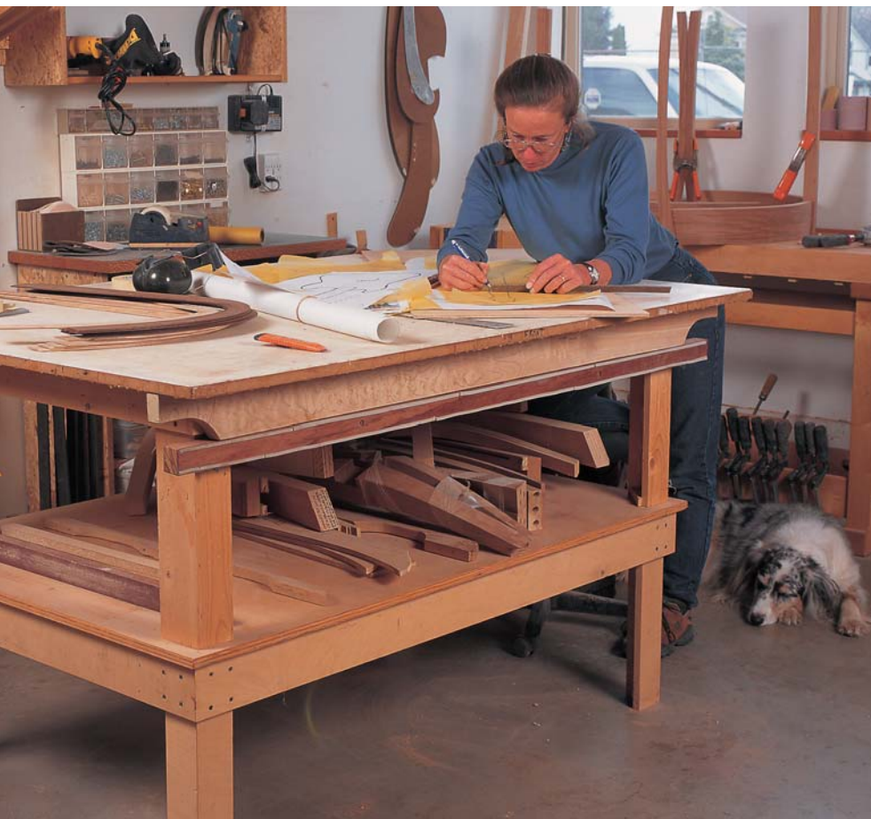
JUDITH AMES'S CENTER WORKBENCH uses the top for drawing, lay-out work, and vacuum-forming curved parts. Once the parts are under pressure, she puts the bag, parts and all, on the shelf below.
