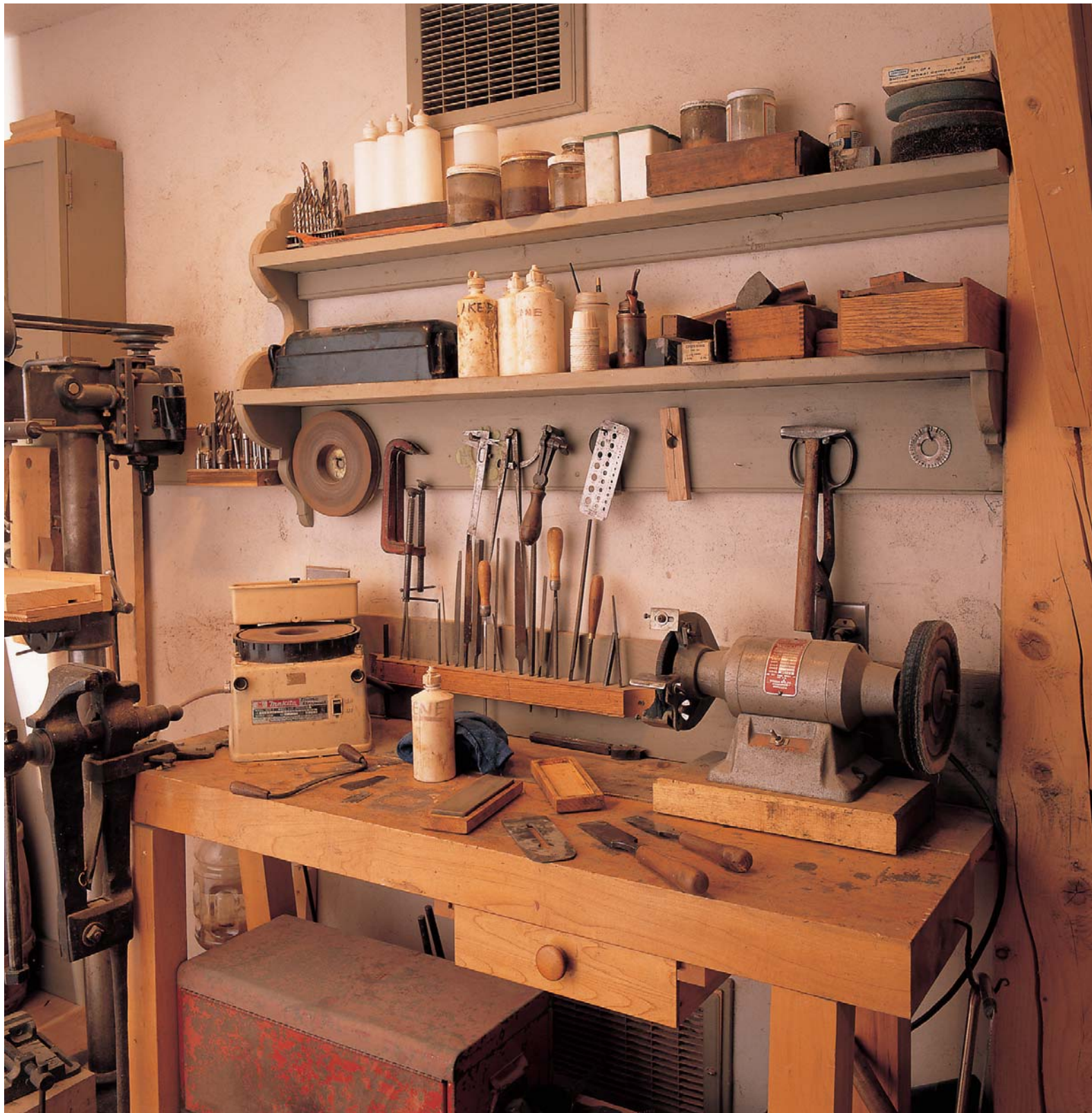
GARRETT HACK'S SHARPENING STATION holds all the basics, including a grinder and sharpening stones. A hand-tool expert, Hack sharpens his handsaws himself and has a saw vise permanently mounted to the bench.
