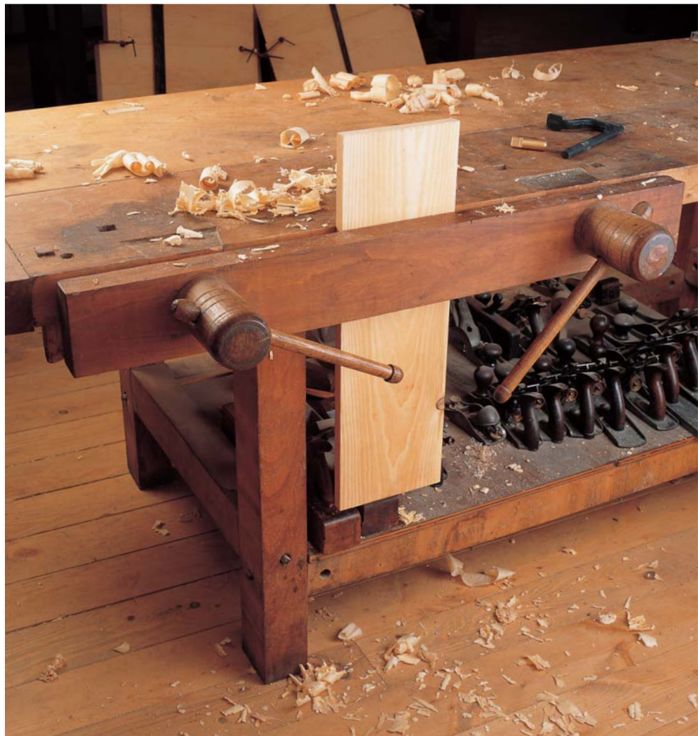
A DOVETAILER'S DREAM , this long double-screw face vise has plenty of room for clamping fairly large panels and holds pieces without racking.
