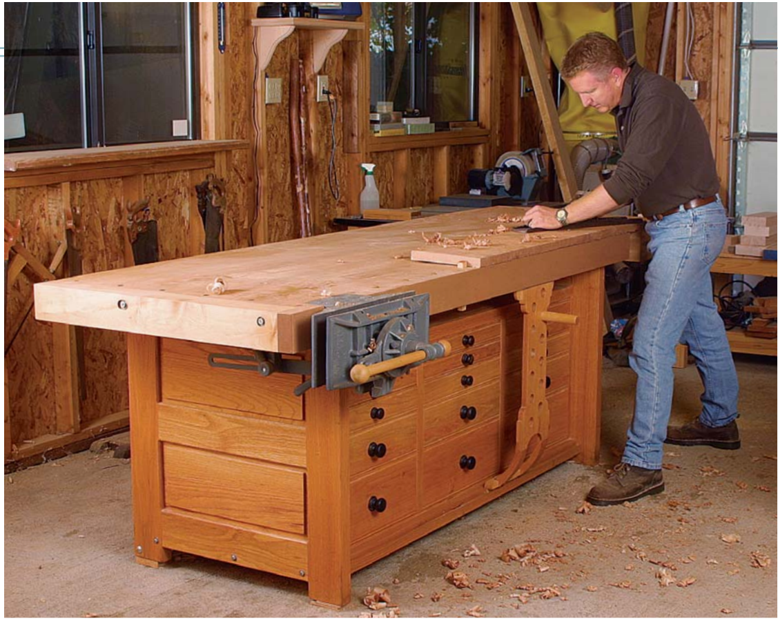
THIS SHAKER-STYLE BENCH built by Jon Leppo features a sliding board jack. The holes accommodate pegs to allow for a variety of board widths. the entire assembly slides back and forth to accommodate boards of different lengths.
