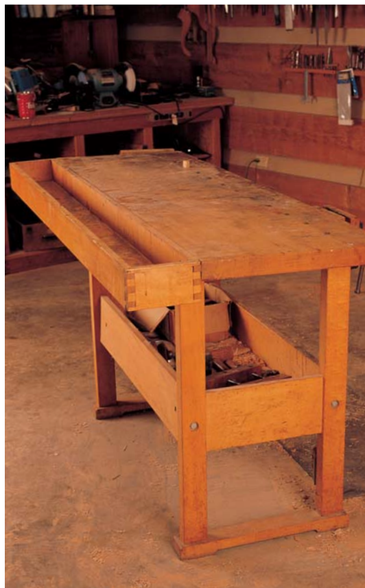
DAVID WRIGHT RETRO-FITTED A TOOL TRAY to a completed bench. He built a simple dovetailed box and attached it to the side of the bench.
