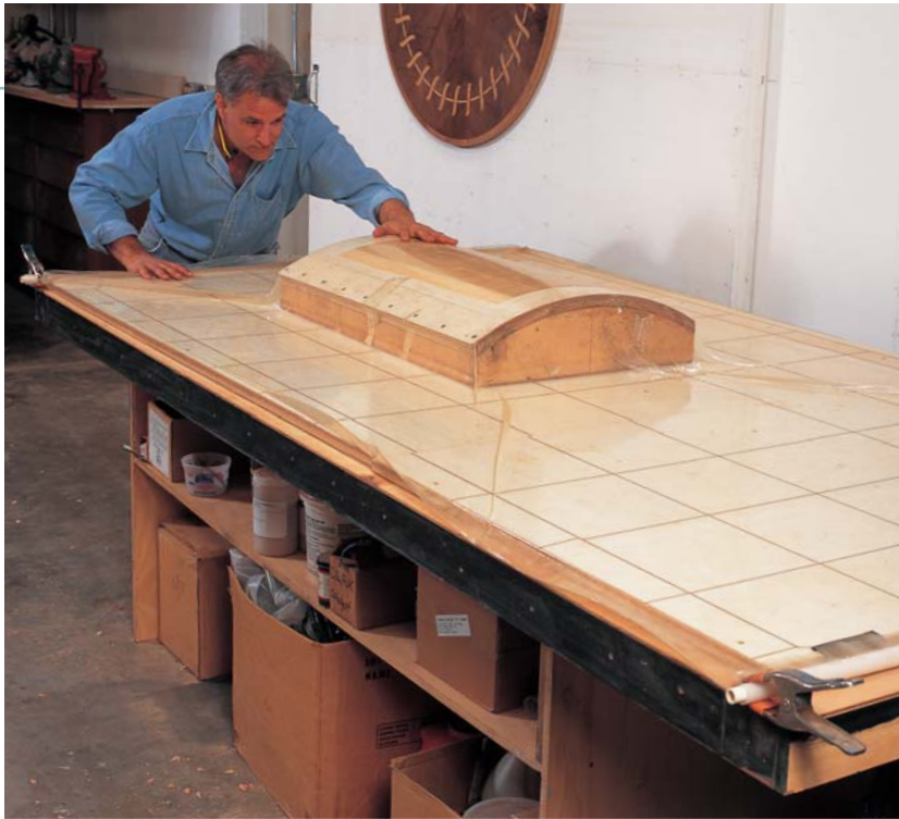
PAUL SCHURCH USES A VACUUM BAG to make many of the curved parts for his furniture. A large smooth surface is essential for proper operation of the bag.
