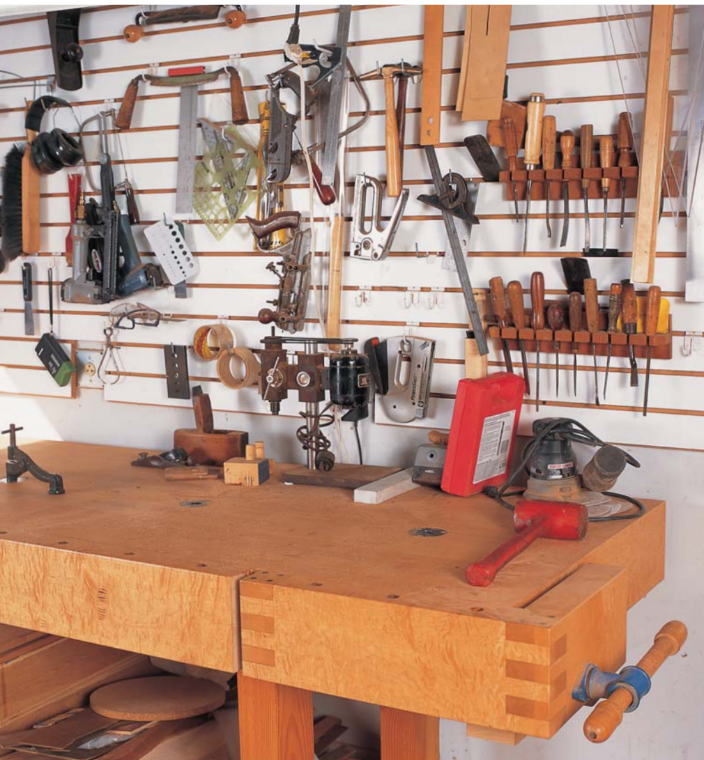
NOT ONLY DOES A TAIL VISE ACT LIKE ANY OTHER end vise in setting the distance between the bench dogs, it excels at tasks like securely holding stock for sawing.
