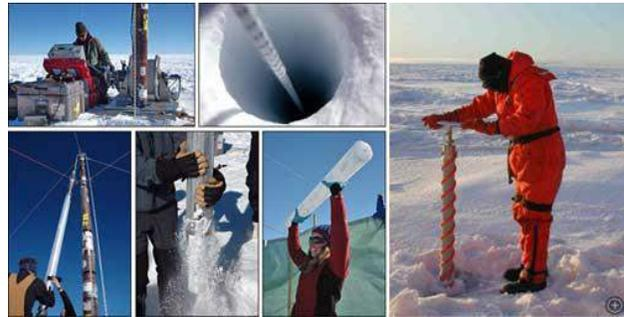
*Clockwise from left: Ice coring machine, hole in ice, pulling ice core from machine, man with hands on ice core tube in ground, scientist holding up ice core, man hand drilling ice core.*
