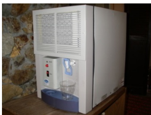
Figure 1: Residential water-from-air machine rated at 7 L/day (mechanical dehumidifier; prototype). Photo by author.
