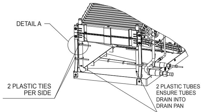
**Step.14d** Next, install the clear plastic tubes which are included in the accessory bag. Ensure the plastic tubes drain into the pan. Also, be sure the clear plastic tubes do not have any restriction. Cutting of the plastic tube is required, please refer to the table for length. Finally, secure the clear plastic tubes to the top drain pan per Detail A. Then to the metal brackets supporting the coil to the top drain pan with the provided plastic ties as shown.
