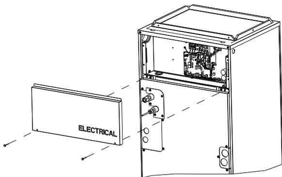
**Step. 3** Remove the panel marked "ELECTRICAL".
