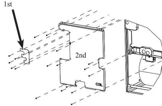
**Step. 4a** Remove the screws securing the (3) panels to the COIL panel shown in the image above. Remove the "1st" panel and "2nd" panel marked "COIL".
