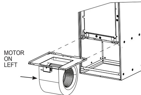
**Step.11** Reinsert the blower assembly with the motor now on the left into the air handler cabinet and reuse the (2) screws that secured the fan assembly in position. Reroute the (2) connectors for the motor back into the enclosure and reconnect.
