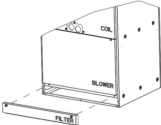
**Step. 1** Remove the panel marked "FILTER".
