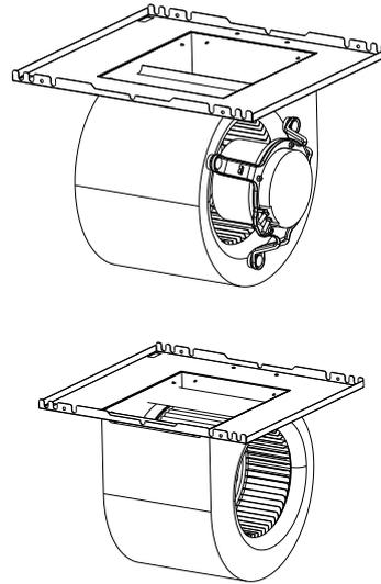
**Step.9** Rotate the blower assembly 180°. The motor should now be on the opposite side
