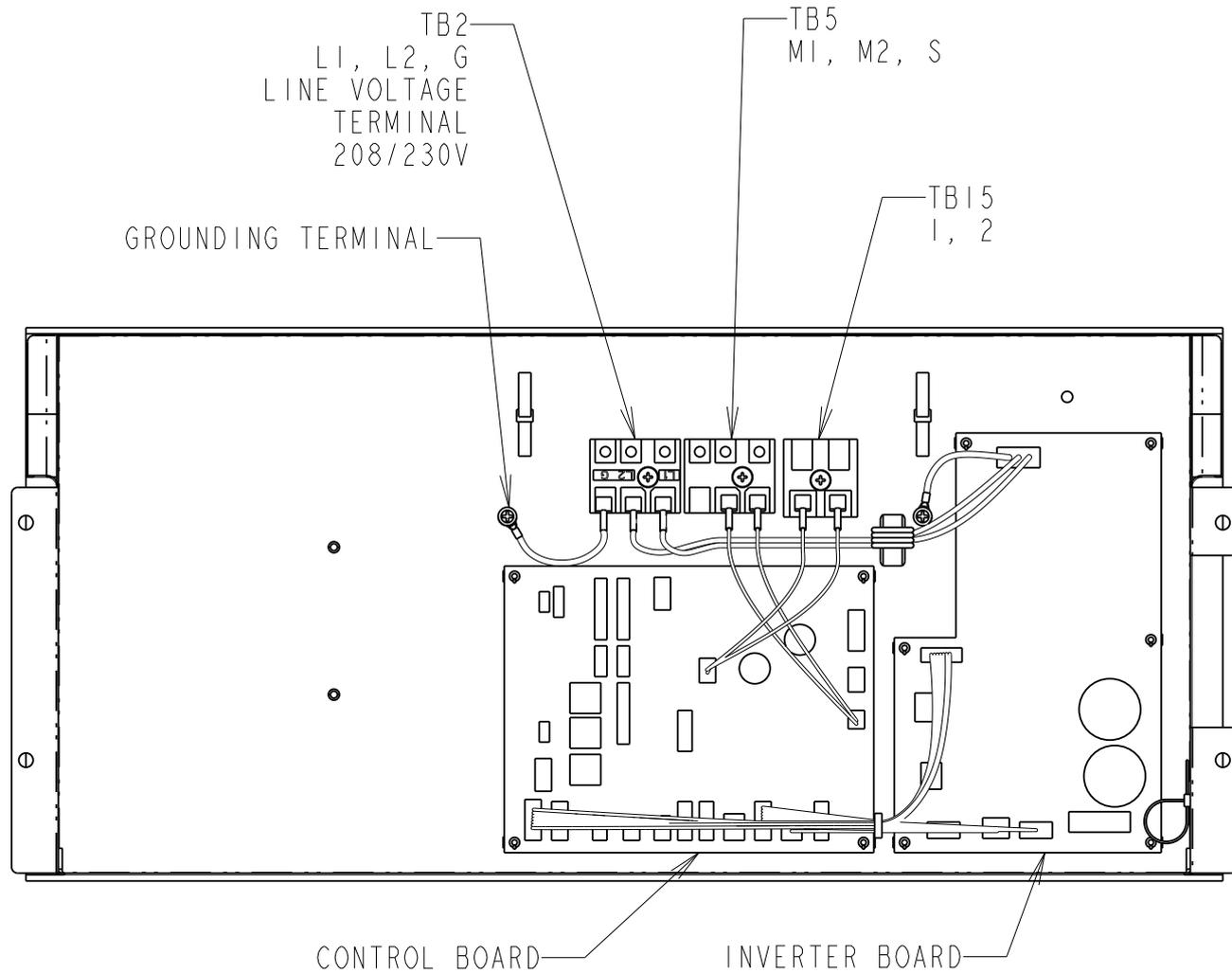
**Connecting remote controller, indoor and outdoor transmission cables**
