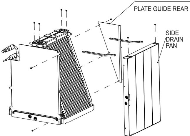
**Step.13** Remove the Plate Guide Rear (3 screws) and Side Drain Pan (4 screws) along with supporting brackets (4 screws) from the coil assembly.
