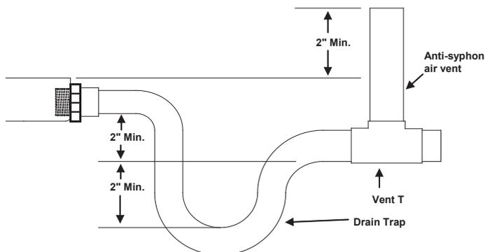
**Note:** Horizontal runs must also have an anti-siphon air vent (standpipe) install ahead of the horizontal run to eliminate air trapping. Horizontal drain lines must be pitched a minimum 1/4" per foot.
