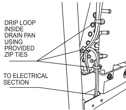
**Step. 4c** In order to prevent water from running down the Thermistor wires into the electrical area, a Drip Loop **MUST** be installed to direct water into the drain pan using the provided zip ties of the accessory bag.
