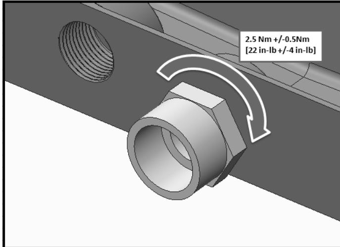
The air handler contains 3/4" FPT drain connections. When the unit is used in the vertical position, there is one set. When the unit is mounted horizontally there is one set. Each set contains a primary drain and a secondary or auxiliary drain. The primary drain is the one that is lowest (even with the bottom of the pan). The secondary drain is at the higher level. They are labeled on the dimensional drawings above.
