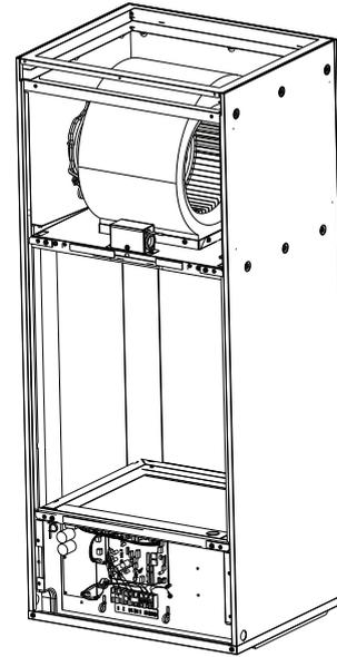
**Step. 3** Rotate the cabinet so the Fan assembly is on top.
