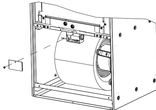
**Step. 5** Remove the electrical enclosure cover mounted on the fan assembly. Disconnect the motor connector along with the connector for the return air thermistor. Remove all of the harnesses from the electrical enclosure leaving only the return air thermistor attached to the electrical enclosure.
