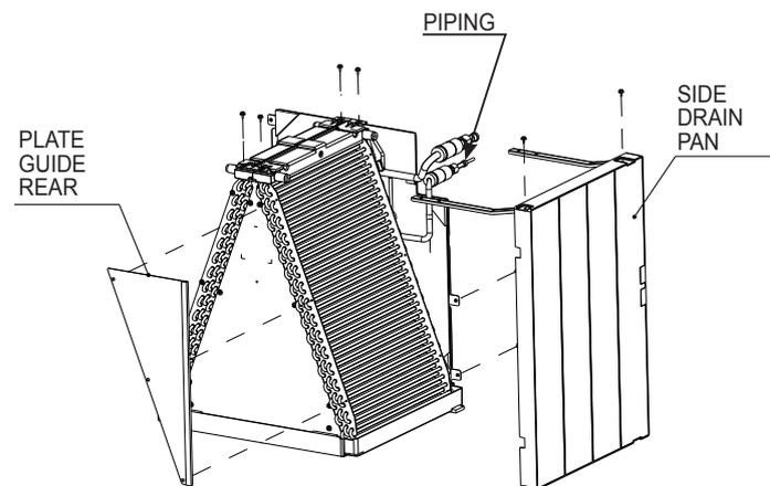
**Step.14b** Reinstall the brackets to the opposite side of the Side Drain Pan. The Side Drain Pan will be reinstalled on the opposite side of the Coil Assembly. Reattach the Plate Guide Rear on the opposite side of the coil assembly.
