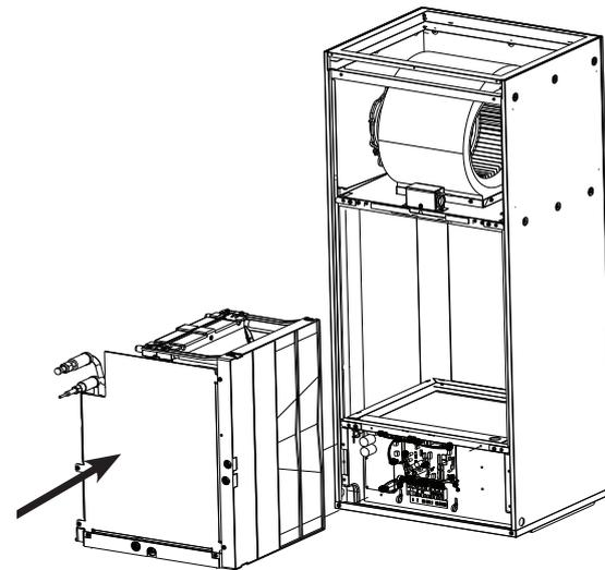
**Step. 4a** Reinsert the coil assembly back into the cabinet. The bracket(s) are not required to be reattached.
