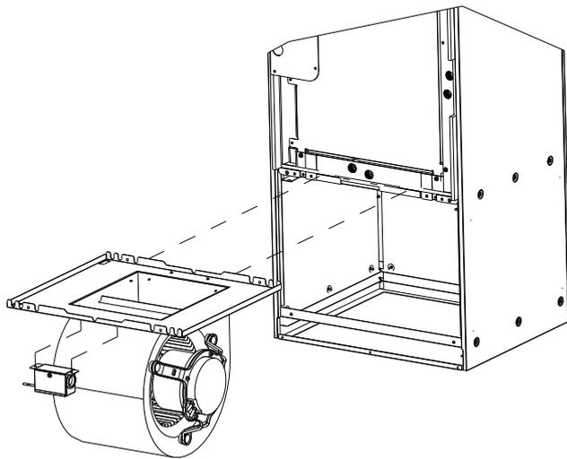
**Step.8** Remove the electrical enclosure from the fan assembly.
