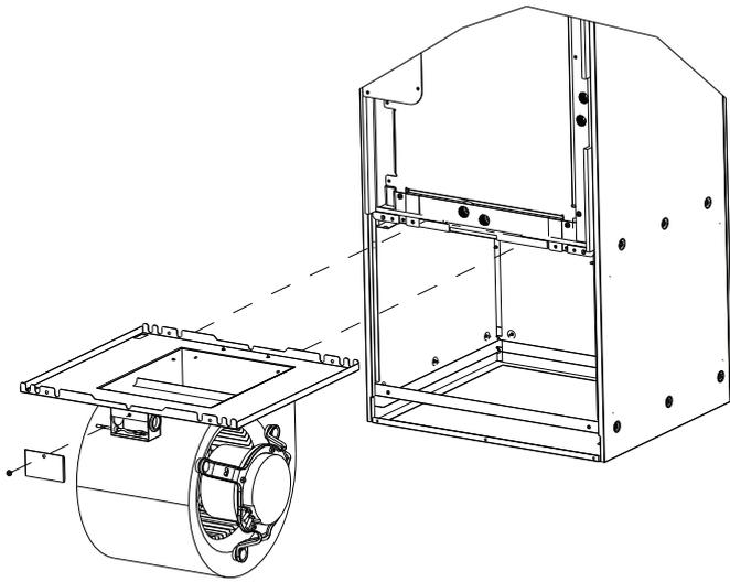
**Step.7** Slide the entire fan assembly out from the cabinet.
