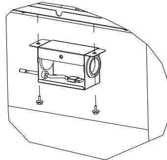
**Step.10** Reinstall the enclosure for the return air temperature sensor on the blower assembly on the opposite side from its original location.
