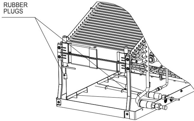
**Step.14c** Remove the rubber plugs indicated in the image above.
