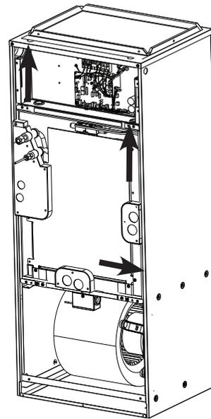
**Step. 4b** Next, remove the smaller panels covering the drain holes and refrigerant lines by first sliding in the direction indicated above.
