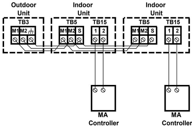
The MA remote controller and the M-NET remote controller cannot be used at the same time or interchangeably.
