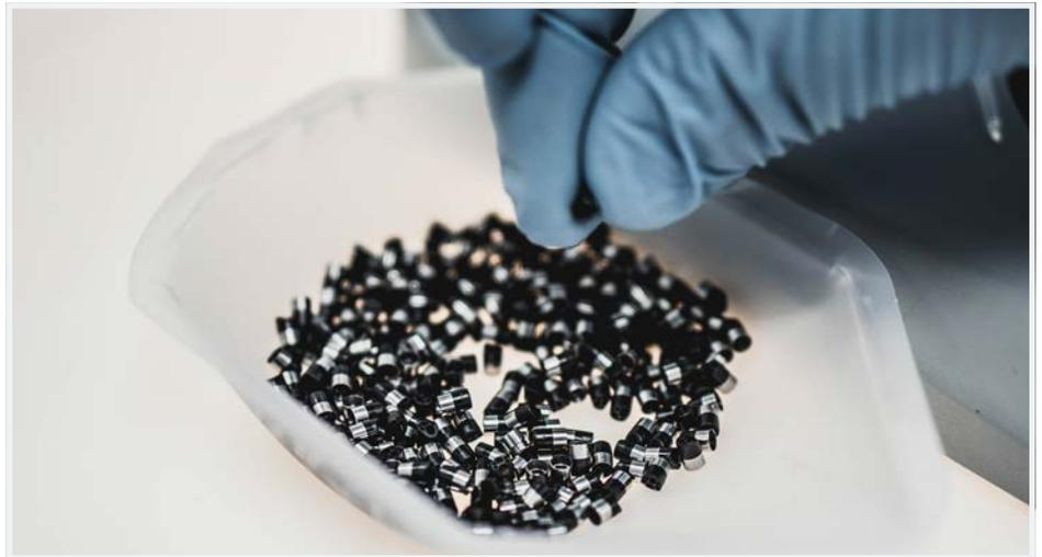
The tip design required extreme micro tooling precision to accomplish the tiny through-holes required for this application. Extremely thin walls in this overmolded tip design measuring .005" at the overmolded section of the metal ring and features +/- .001" tolerances throughout were enabled by micro injection molding technology.
