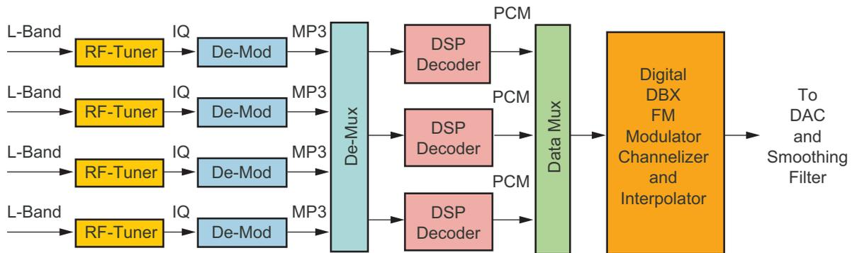
Figure 2 – High-level block diagram of transceiver
