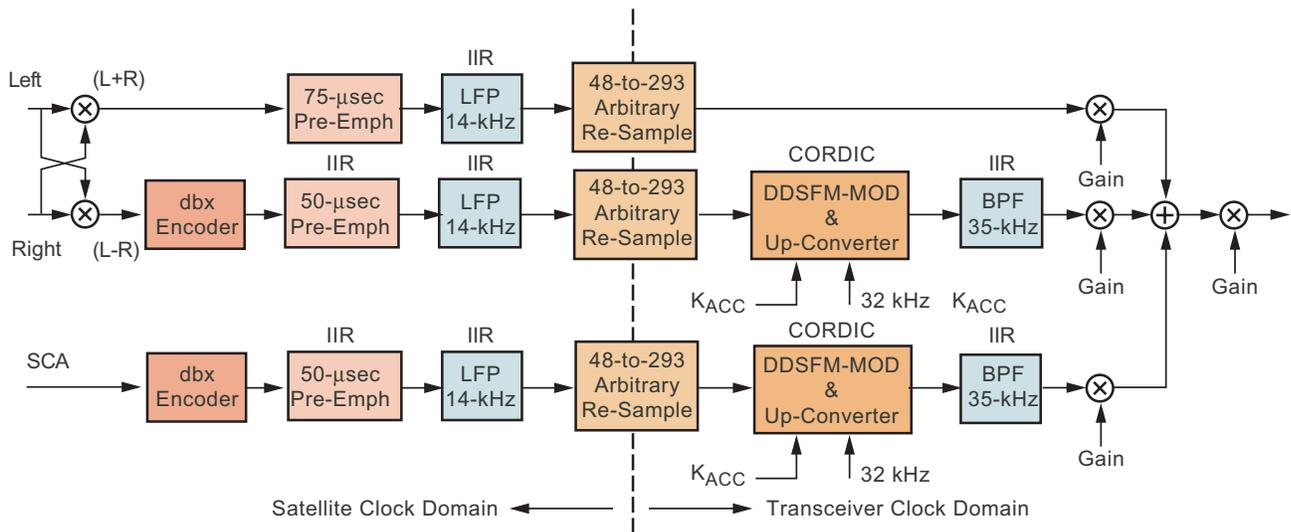
Figure 5 – Block diagram of single-channel processing block: stereo and SCA signal
