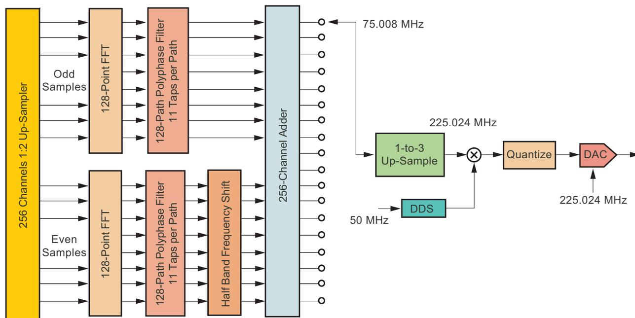
Figure 6 – Polyphase channelizer and final post-processing tasks to operate output DAC
