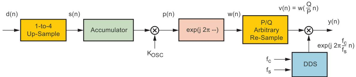
Figure 4 – Signal flow diagram: DSP-based complex baseband FM modulator
