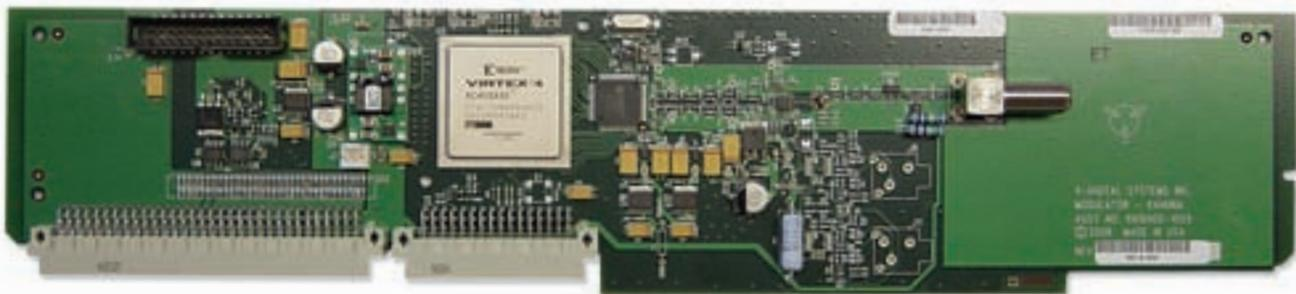
Figure 7 – Re-modulator board showing Xilinx Virtex-4 FPGA that implements 384 FM modulators implemented on 192 modulator boards in the equipment bay shown in Figure 1.
