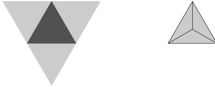
Figure 3.2: On the left an equilateral triangle divided into 4 equilateral triangles of side a . Folding the three outside equilateral triangles to join their tips produces the figure in the right which is a tetrahedron seen from above.
