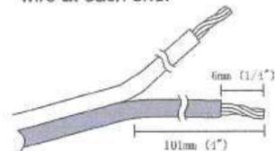
3. Using a wire stripper, remove about 1/4" (6mm) of insulation from each wire. Then twist the ends of each wire.
