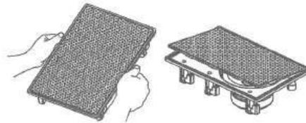
Carefully remove the dust cloth from behind the grill and replace it after you are finished painting.
