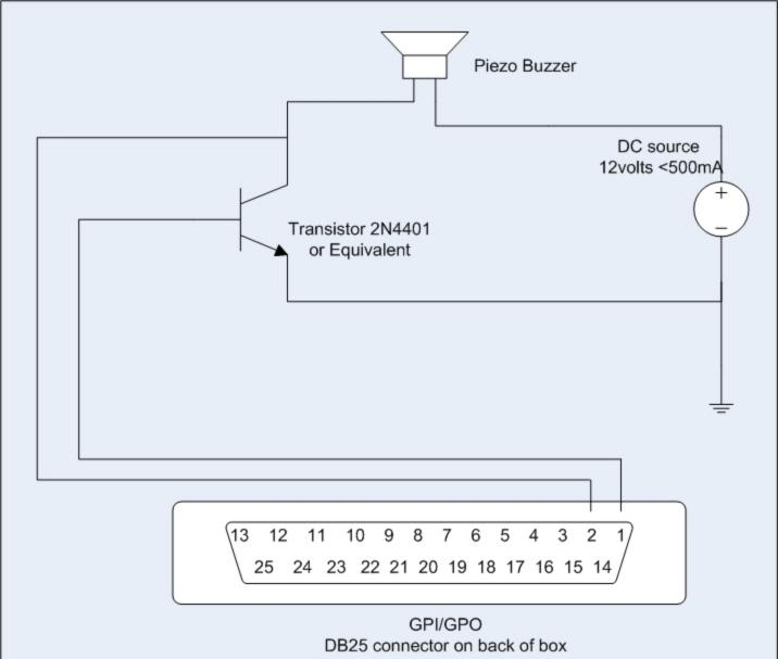
Note: This is a simple circuit that will sound a buzzer each time a network message is received.
