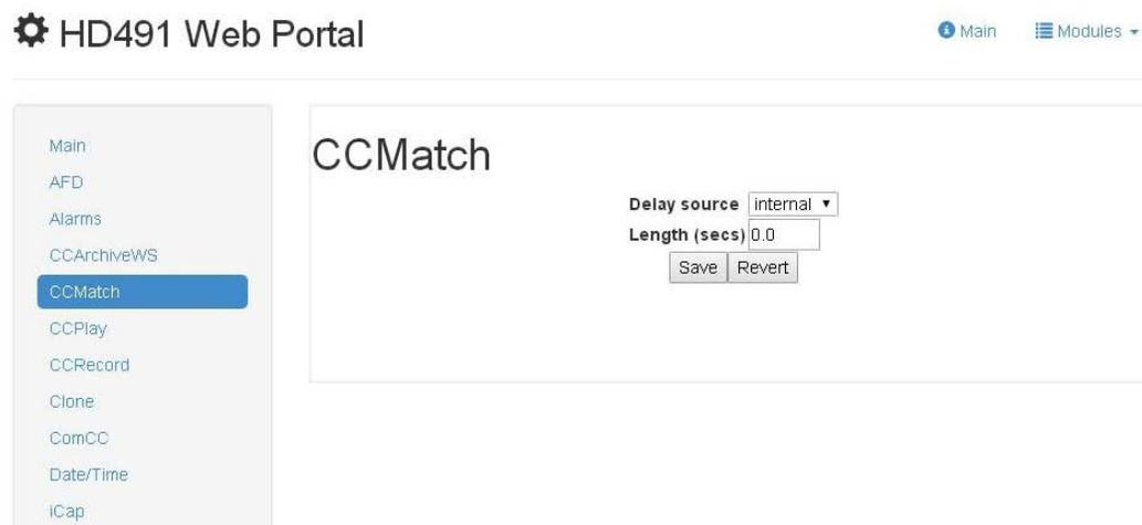
In HD491 Build versions 2.5.3 and higher, and all HD492 encoders, CCMatch contains additional options as shown in Figure 4 and described below.
