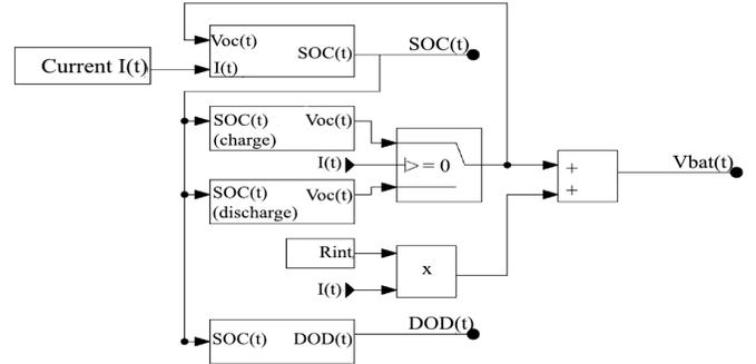
Fig. 2. Diagram of the block model of the state of charge battery
