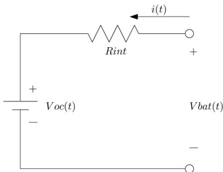
Fig. 1. Circuitual Diagram of the Theoretical Model
