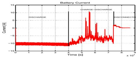
Fig. 3. Current Charge-Discharge of the First Case Study
