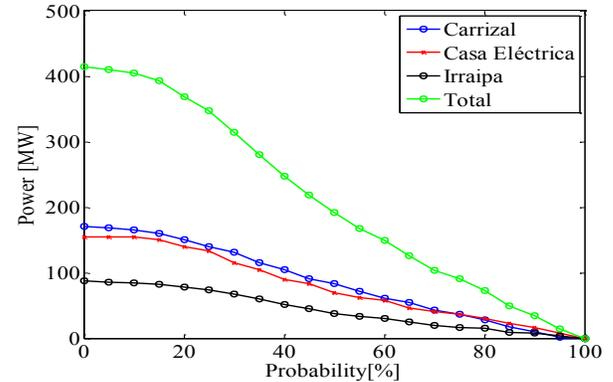
Figure 3. Cumulative probability function of the power produced by the three wind power plants in one hour.
