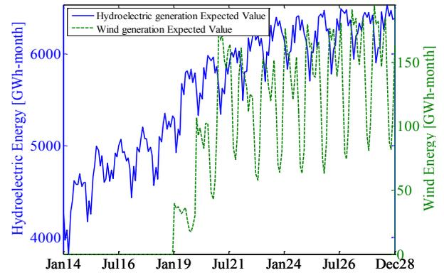
Figure 1. Expected value of the power generation from wind and hydraulic power plants. Complementarity.
