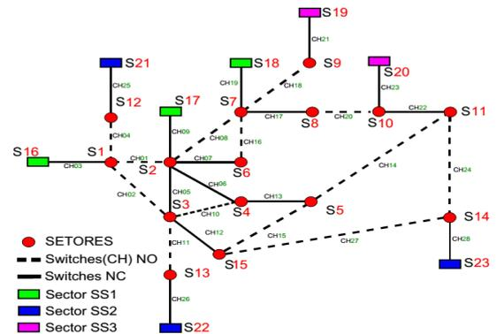
Figure 2 - Validation System in Sector Representation where "SS" are Substations.
