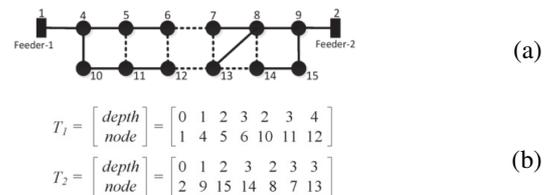
Figure 1 – a) A distribution system with two feeders modeled on graphs with two dispersion trees; b) NDE vector graph Forest of Figure 2a. [10].
