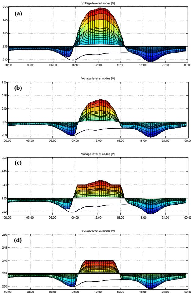
Figure 7: Simulated voltage levels at nodes in the rural grid, with uncontrolled feed-in (a), with controlled battery charging (b), with power factor adjustment (c), and with a combination of both (d)
