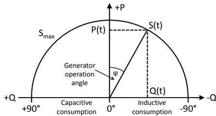
Figure 3: Inductive and capacitive reactive power [2]
