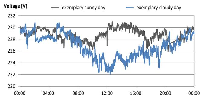
**Figure 1: Voltage level during sunny and cloudy days; low voltage node in an urban power grid**
