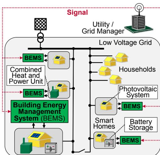
Figure 2: Visualization of a future energy system combining decentralized BEMS to supply grid services
