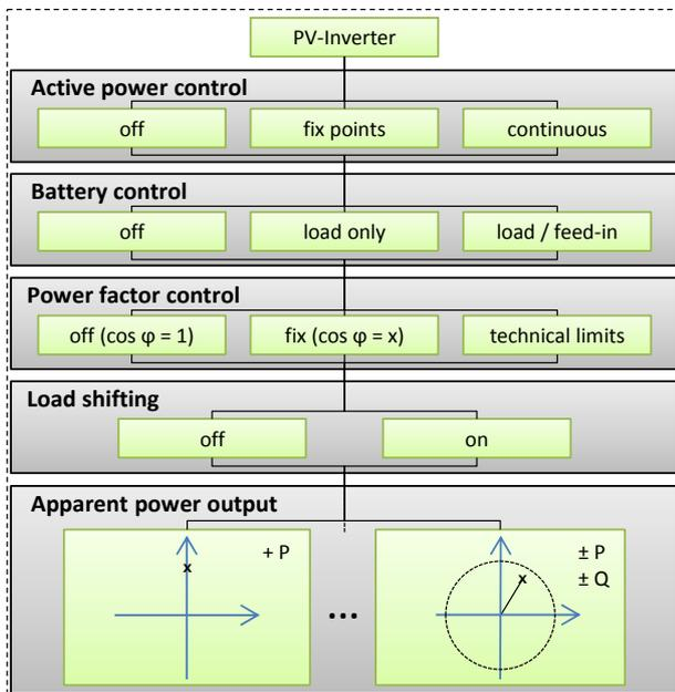
Figure 4: Setup specifications and control schemes
