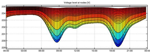
Figure 6: Simulated voltage levels at nodes in the rural low voltage grid
