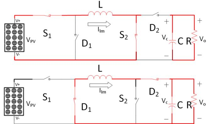
Figure 2. Non-inverter Buck-Boost DC-DC converter operational states.
