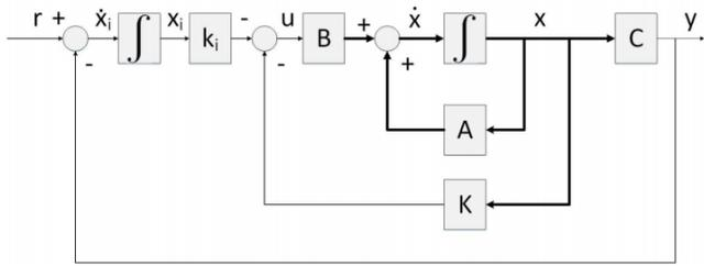
Figure 3. Stead-space feedback closed loop control with reference input and integral action.
