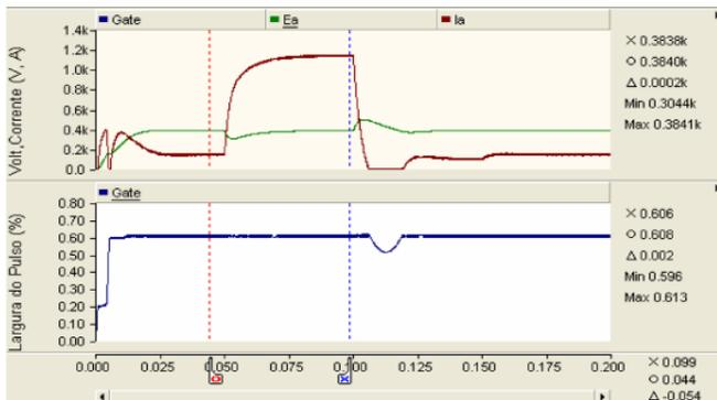
Figure 9. Voltage control sensibility of parasite resistances and inductance: output voltage (green); output current (red); and duty cycle (blue).
