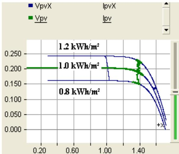
Figure 12. PV power plant operating at MPP: PV output voltage (green), PV I-V curve for different solar irradiance levels (blue).
