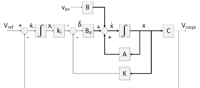
Figure 4. Block diagram of steady-space control method related to DC-DC power converters.
