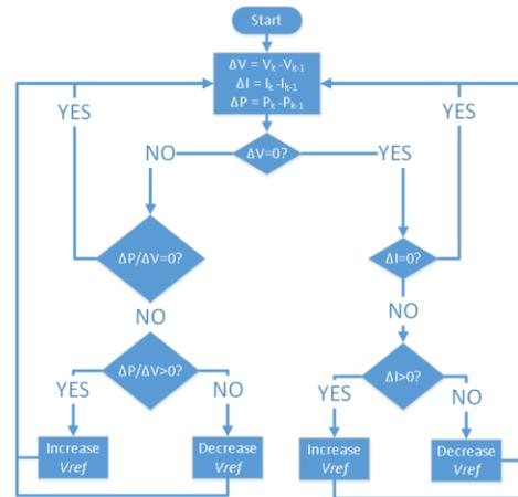
Figure 5. Incremental Conduance (IC) algorithm flowchart.
