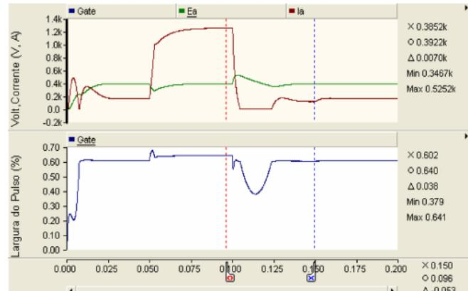
Figure 8. Voltage output control scheme considering load steps: output voltage (green); output current (red); and duty cycle (blue).
