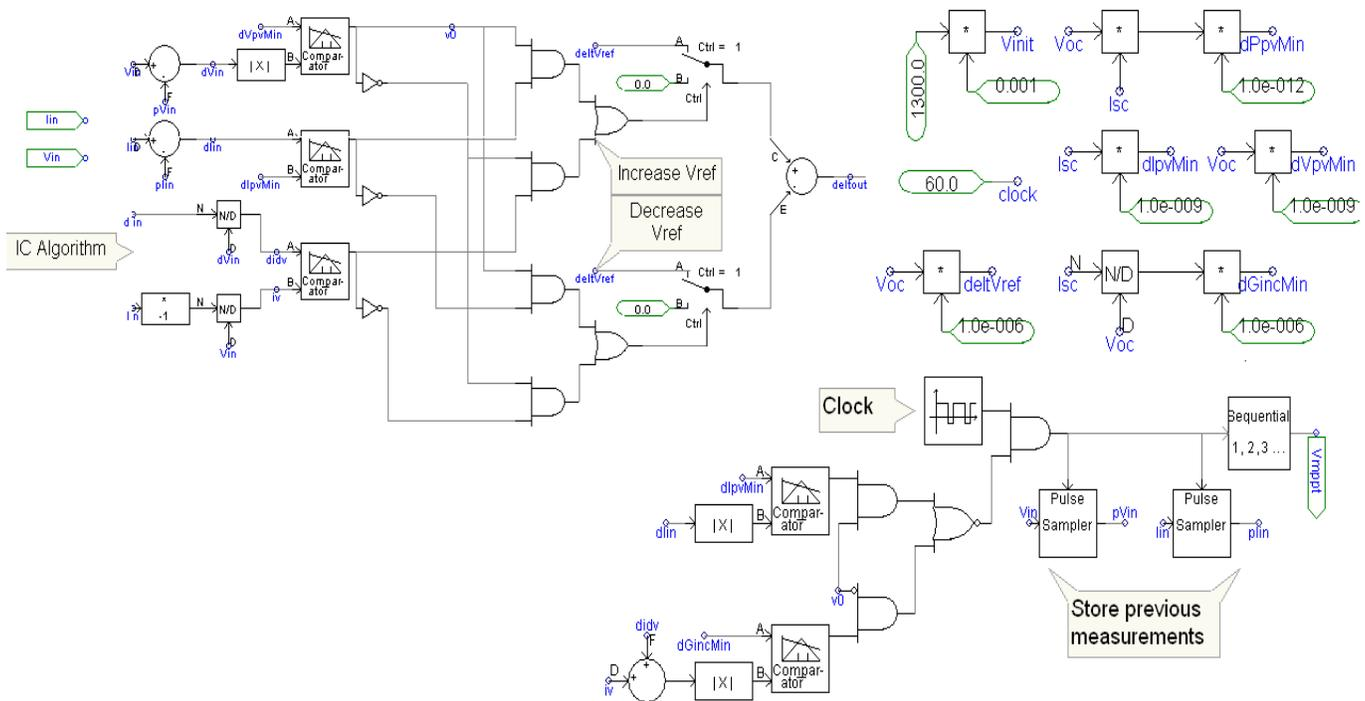
Figure 10. Implementation of the IC algorithm at PSCAD.
