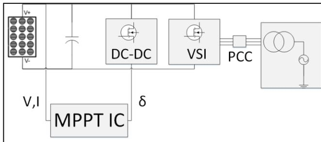
Figure 6. Grid-tie PV system with MPPT schema.
