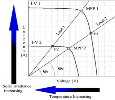
Figure 1. Effects on curve V-I of solar cells considering increases of temperature (to left) and irradiance (to up).
