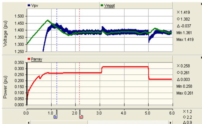
Figure 11. Output PV voltage control using non-inverter Buck-Boost converter under MPP: PV output voltage (blue); MPPT output reference voltage (green); PV output power (red).
