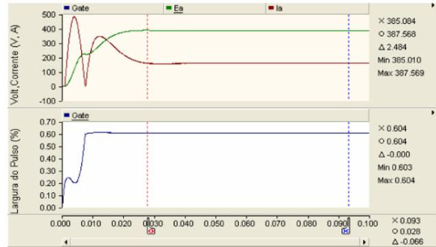
Figure 7. Output voltage control of non-inverter Buck-Boost converter: output voltage (green); output current (red); and duty cycle (blue).
