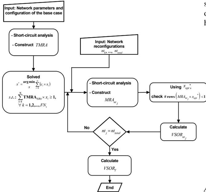
Figure 1. Proposed method to assess the impact of the DNR on the OPP of voltage sag monitors
