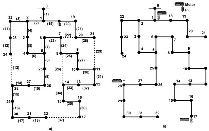
Figure 2. a) One-line diagram, b) Optimal placement of voltage sag monitors
