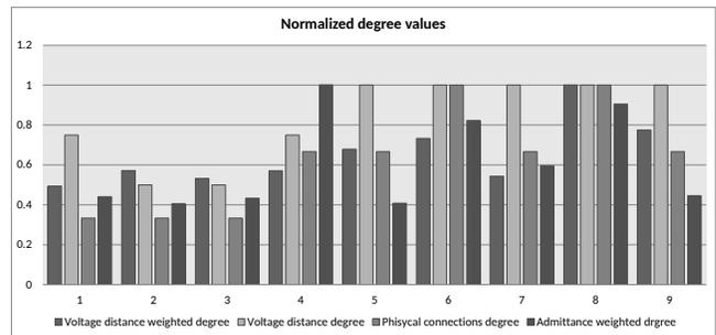
Fig. 3: Normalizes degree centrality measures for the WSCC 9 bus system.
