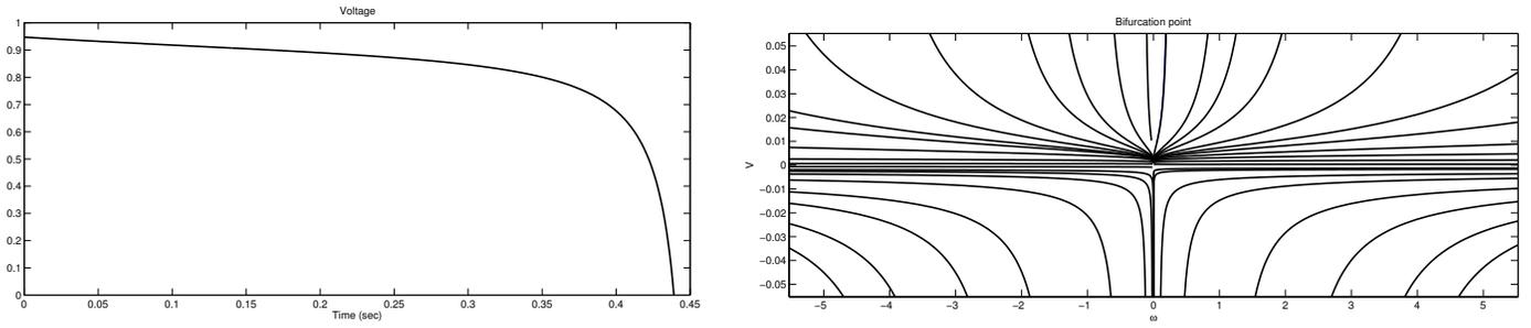
Fig. 1: *Left.* Voltage collapse for a tree bus system in bifurcation point obtained from variations in reactive load  $\mu$ . *Right.* Phase plane at the point of bifurcation. Simulation parameters from model proposed in [7].
