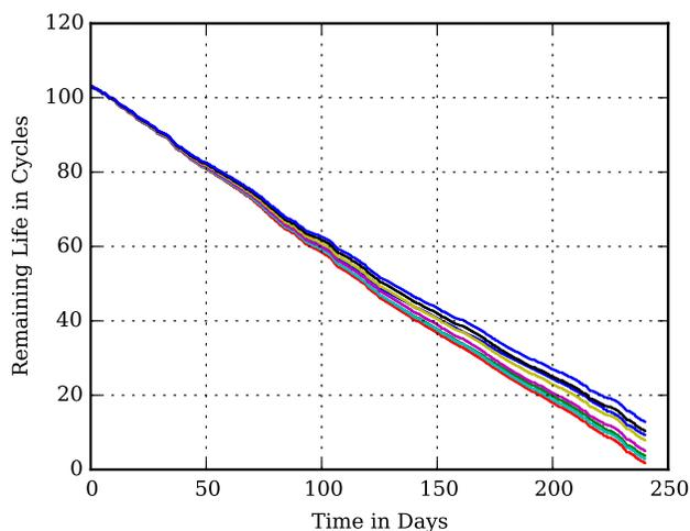
Figure 2. Remaining life of the crisp strategy for different battery capacities taking as the maximum power ratio of the storage system half of the capacity. For the fuzzy and perfect information strategy there is no difference on the life remaining if the power to capacity ratio is constant.
