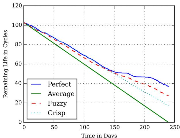
Figure 1. Remaining life of the storage system in terms of cycles. The initial value of the remaining life cycles are 103 cycles, and for the average strategy the remaining life is less than 1 cycle.
