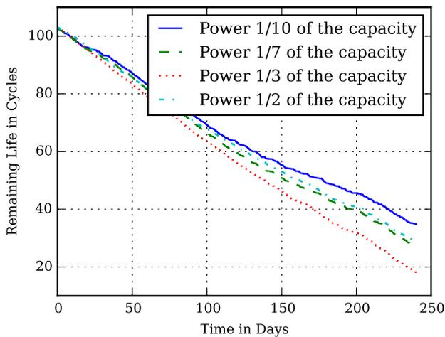
Figure 3. Remaining life for the fuzzy logic strategy for different maximum charge/discharge power ratio for the reference capacity.
