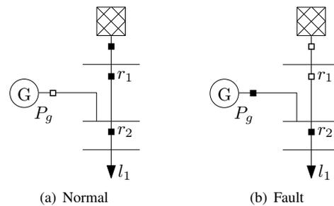
Fig. 1. Operation of a distribution system with DG. a) Distribution system when the main grid is available. b) Isolated operation when a fault event arises.
