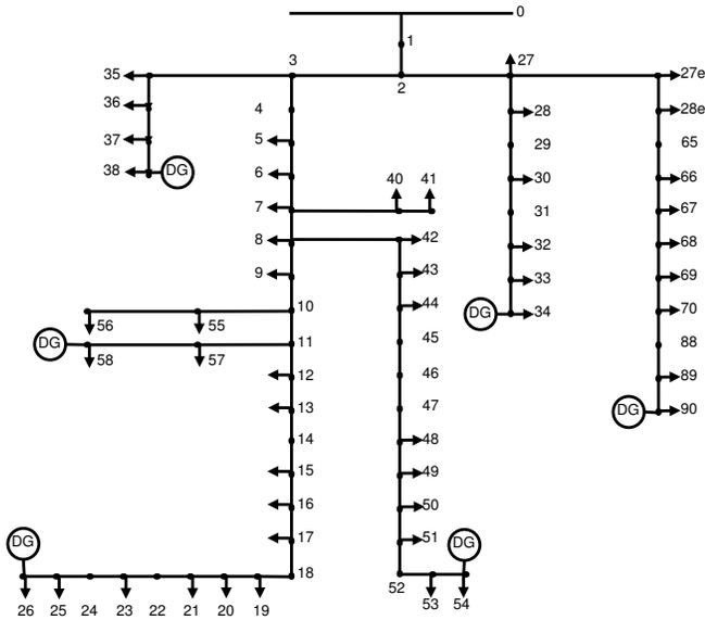
Fig. 4. 70-nodes test feeder with DG penetration, adapted from [19].
