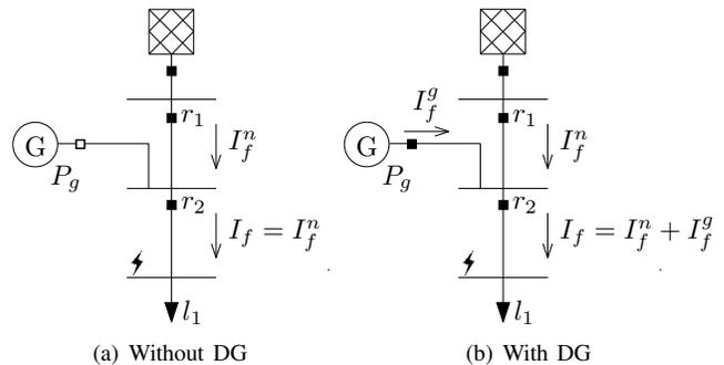
Fig. 2. Short circuit currents in a distribution system. a) Short circuit in a traditional system. b) Short circuit in a DG-enhanced feeder.
