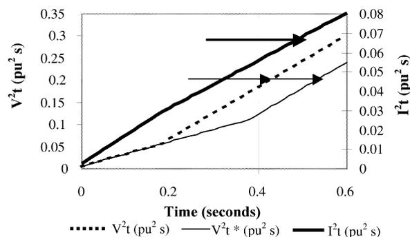
Fig. 9, Comparison of overcurrent and SE Specific Energies.
