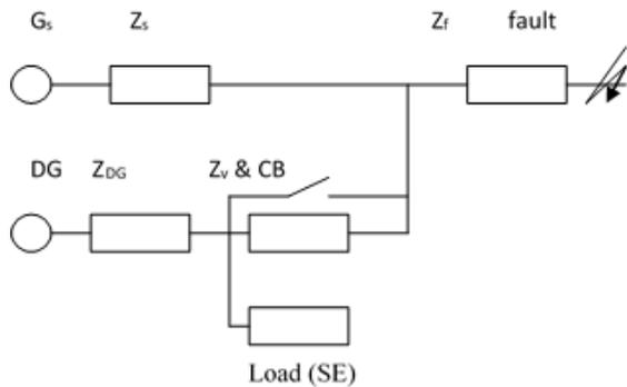
Fig. 2, Simplified distribution system with a distributed generator.
