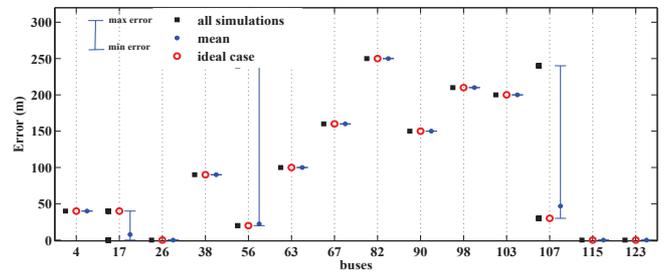
Fig. 13. Errors in fault location with  $\pm 50$  errors in loads - uniform distribution.
