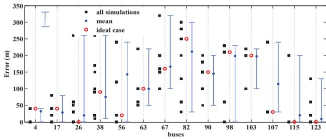
Fig. 7. Errors in fault location with errors in measurements - normal distribution.
