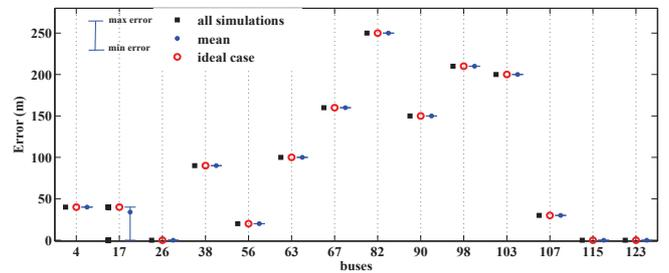
Fig. 12. Errors in fault location with  $\pm 50$  errors in loads - normal distribution.
