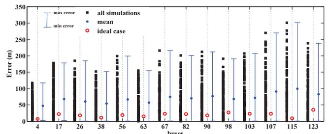
Fig. 4. Errors in fault location with errors in measurements - uniform distribution.
