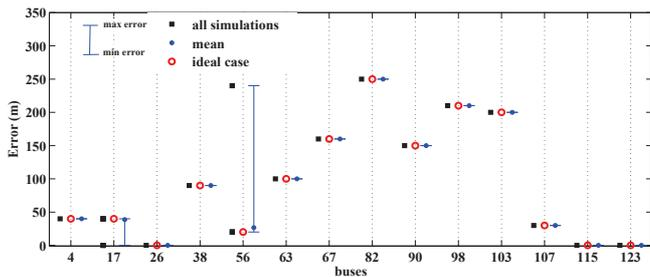
Fig. 9. Errors in fault location with errors in line parameters - normal distribution.
