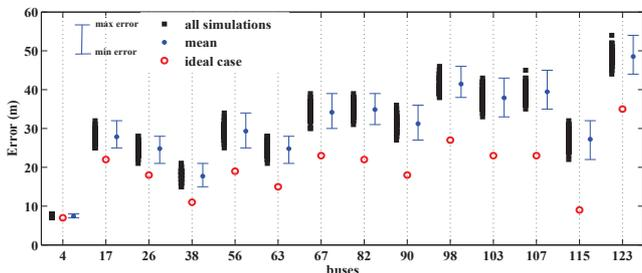
Fig. 5. Errors in fault location with errors in line parameters - normal distribution.
