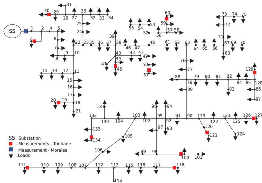
Fig. 2. Real power distribution system (134 nodes).
