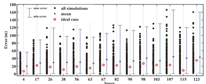
Fig. 3. Errors in fault location with errors in measurements - normal distribution.
