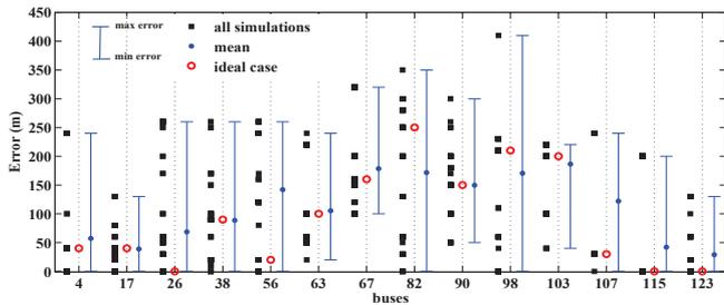
Fig. 8. Errors in fault location with errors in measurements - uniform distribution.
