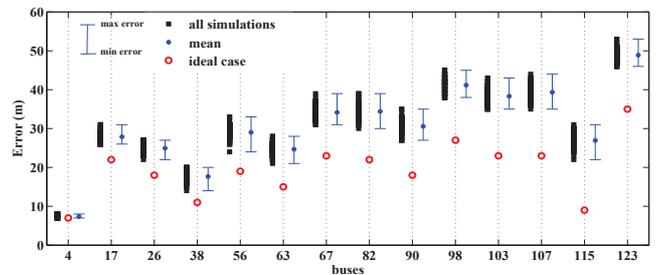
Fig. 6. Errors in fault location with errors in line parameters - uniform distribution.
