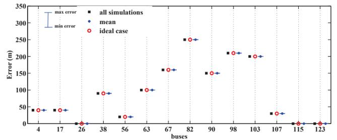
Fig. 11. Errors in fault location with  $\pm 20$  errors in loads - normal distribution.
