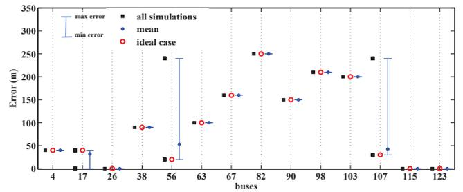
Fig. 10. Errors in fault location with errors in line parameters - uniform distribution.
