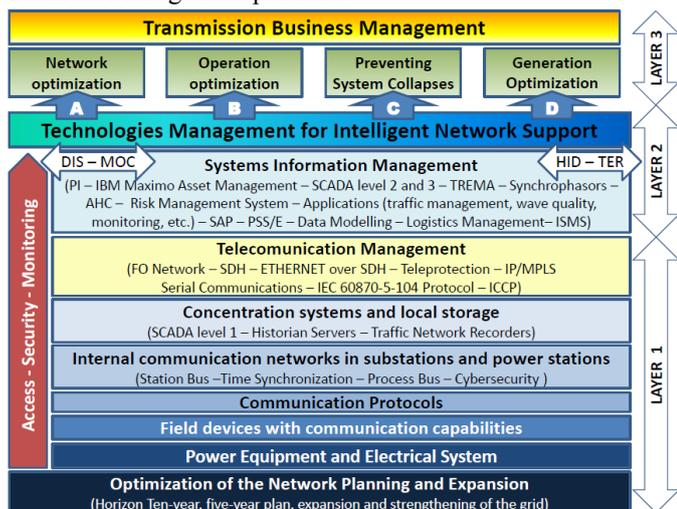
Figure 4. Transmission Network Smart Grid model.
