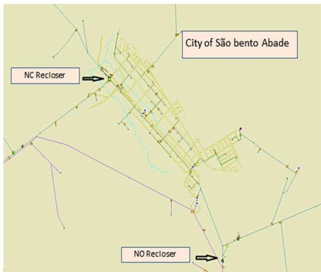
Figure 4. Topology with 1 NC recloser + 1 NO recloser, supplying the City of São Bento do Abade-MG.
