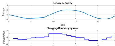
Figure 5. Battery storage capacity and charging/discharging rate along the day.
