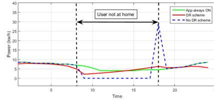
Figure 4. Power consumed from the grid by an end-user in the different schemes.
