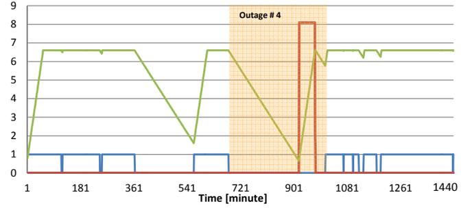
Fig. 5: Baseline management results: blue is outage signal (1 means grid-connected time, 0 means outage time), green is SOC  $[kWh]$ , red is diesel generation  $[kW]$ .
