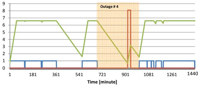
Fig. 7: PMS results: blue is outage signal, green is SOC [kWh], red is diesel generation [kW].
