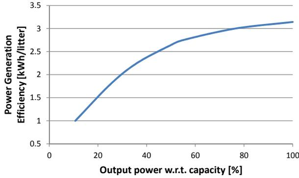
Fig. 2: Diesel efficiency characteristic curve
