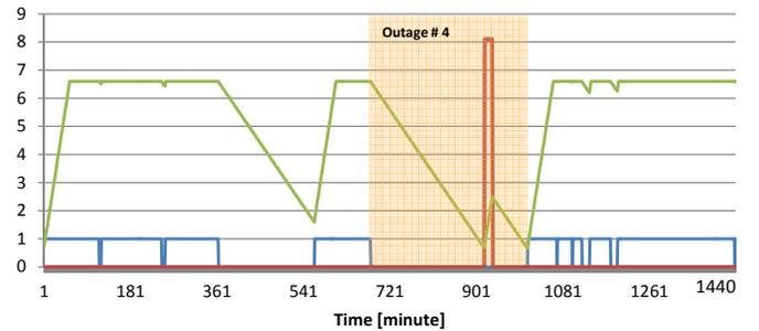
Fig. 6: Ideal management results: blue is outage signal (1 means grid-connected time, 0 means outage time), green is SOC  $[kWh]$ , red is diesel generation  $[kW]$ .
