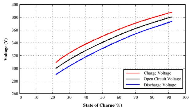
Figure 1. Battery open circuit voltage measured from an experiment.
