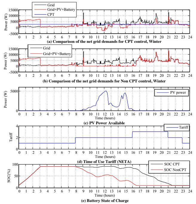
Figure 3. Example simulation results in winter: (a) Community grid demand with *CPT*, (b) Community grid demand without *CPT*, (c) PV power available, (d) Time of use tariff, (e) Battery state of charge.
