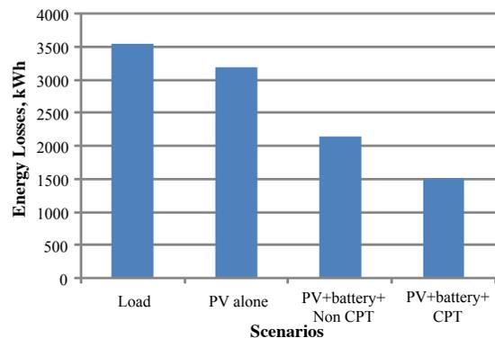
Figure 6. Total transmission line energy losses during the peak period for four scenarios over 12 years.
