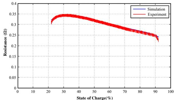
Figure 2. Battery internal resistance Vs state of charge.
