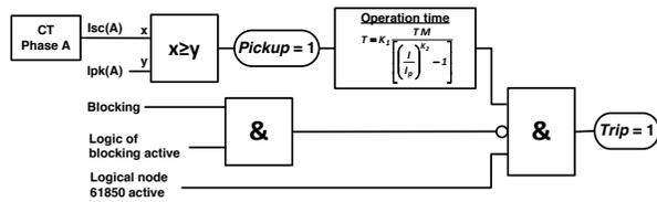
Fig. 2. MBR model of time overcurrent relay – phase A.
