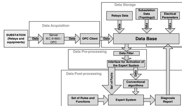
Fig. 1. Functional diagram and flow of the automation system data
