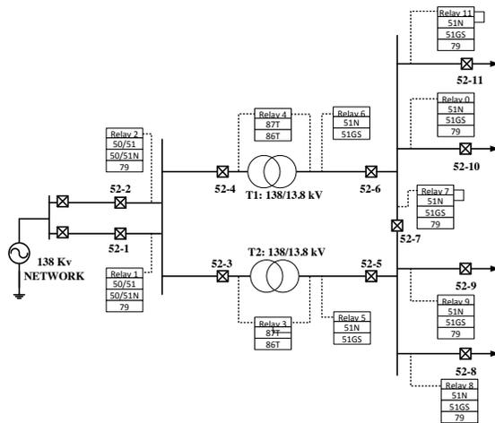
Fig. 6. Topology of the substation
