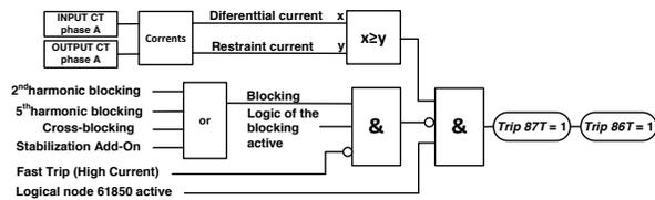
Fig. 4. MBR Model of differential protection – phase A
