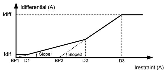
Fig. 3. Differential protection operation curve
