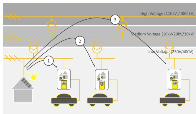
Figure 1: Overview of SyncFuel's EV interconnection setups with involvement of various grid levels
