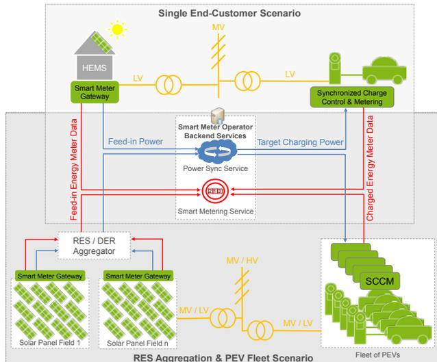
Figure 5: ICT Concept for remotely synchronized Own-Consumption for Single and Fleet PEV Charging Scenarios
