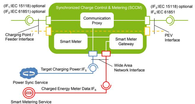
Figure 4: Concept overview of the Synchronized Charge Control & Metering (SCCM)
