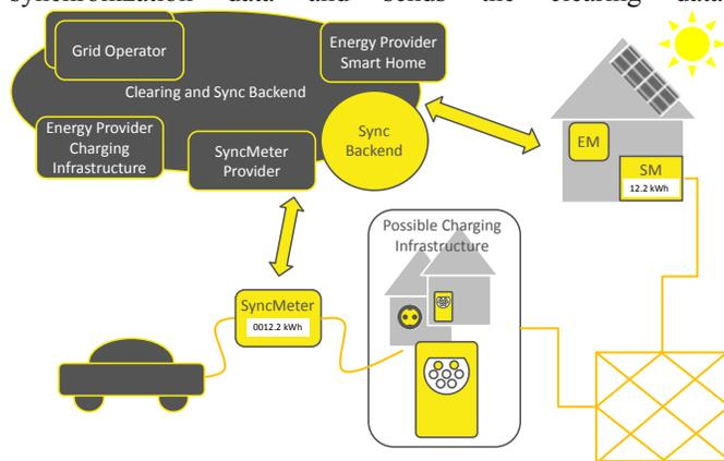
Figure 2: Technical concept of the SyncFuel approach
