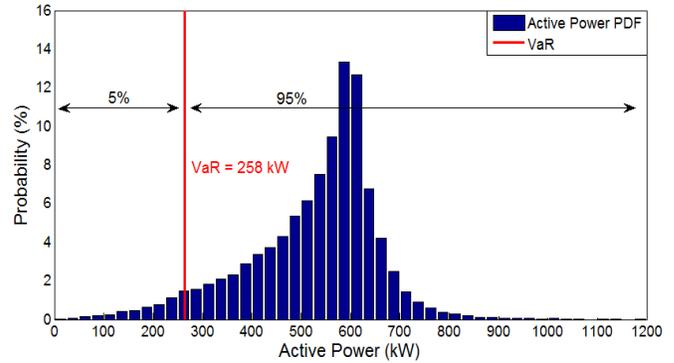
Figure 1 – Power dispatched by DGs (january – 4 a.m.) and its VaR value.
