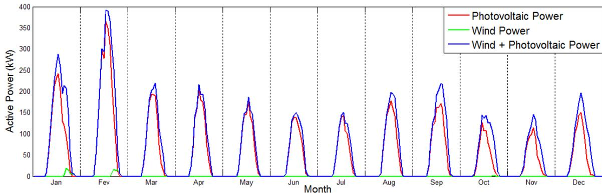
Figure 2 – Annual firm capacity curve of DGs.
