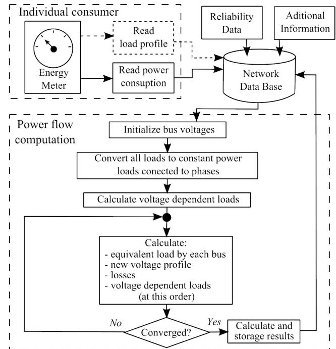
Fig. 2: Power flow computation process
