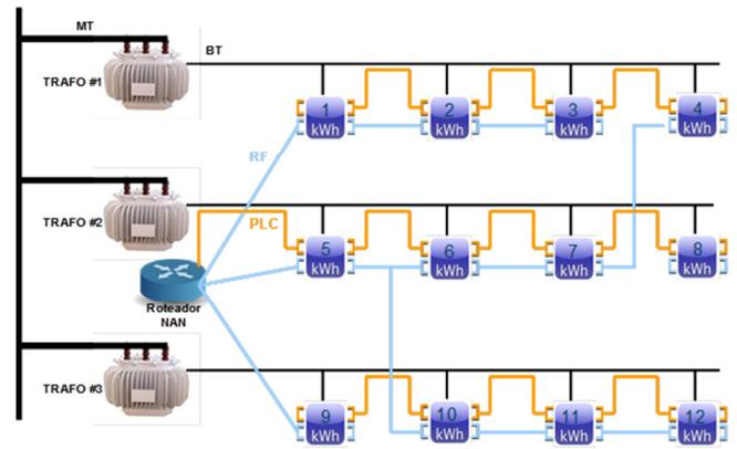
Figure 1. PLC crossing transformers through RF bridges.
