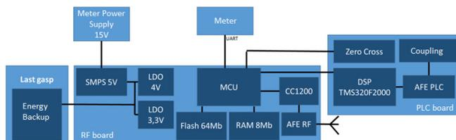
Figure 2 - Diagram of the communication module blocks.
