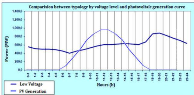
Fig. 2. Comparison between load typology by voltage level and photovoltaic curve
