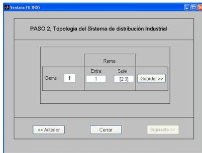
Figure 1 Window 2, allows entering each bus and branch coming in out (construction of incidence matrix).
