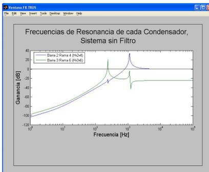
Figure 3 Resonance frequency of each capacitor, system without filter.
