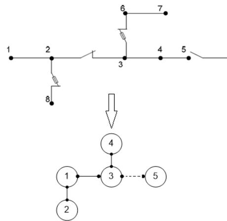
Figure 1. Areas delimited by switches on a distribution network
