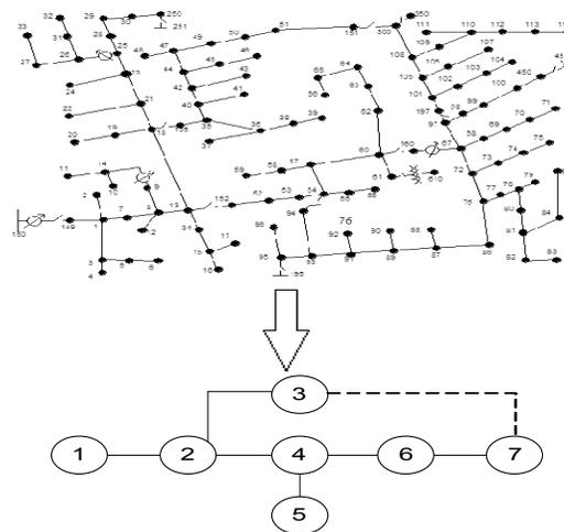
Figure 2. Original IEEE 123-node and its respective graph
