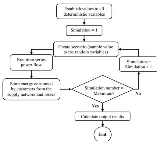
Figure 1. Flowchart of the Monte Carlo based algorithm
