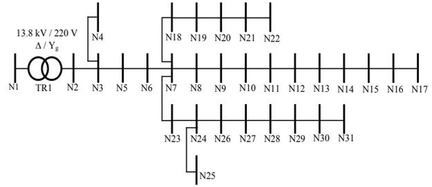
Figure 2. Test network schematic.
