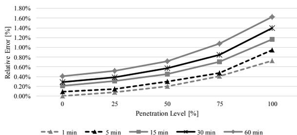
Figure 8. Relative error of energy supplied for 1-year horizon (case 2).
