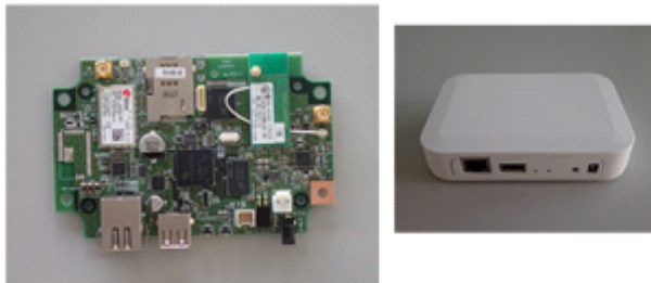
Fig. 3. Digital Grid Controller
