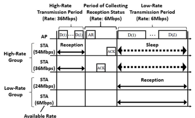
Fig. 1. Multi-rate parallel multicast transmission for power saving.
