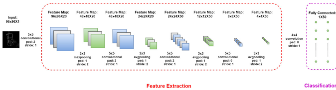
Fig. 4. An illustration of the architecture of our CNN classifier
