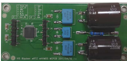
Fig. 4. Photo of the test board with the packaged pulser.
